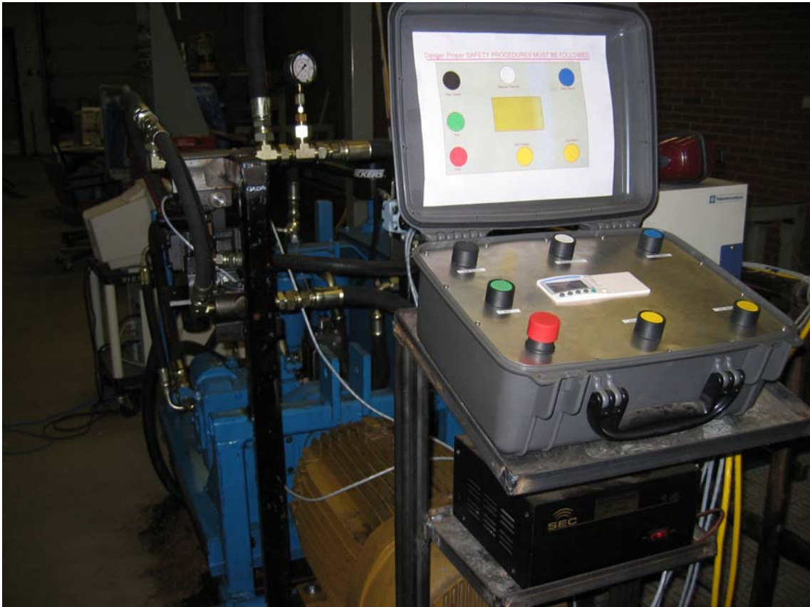
Figure 3.4 Electronic control box to control carriage movement
