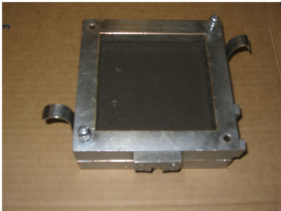
Figure 3.10 Reduction in height of soil sample after applying load by the hydraulic jack
