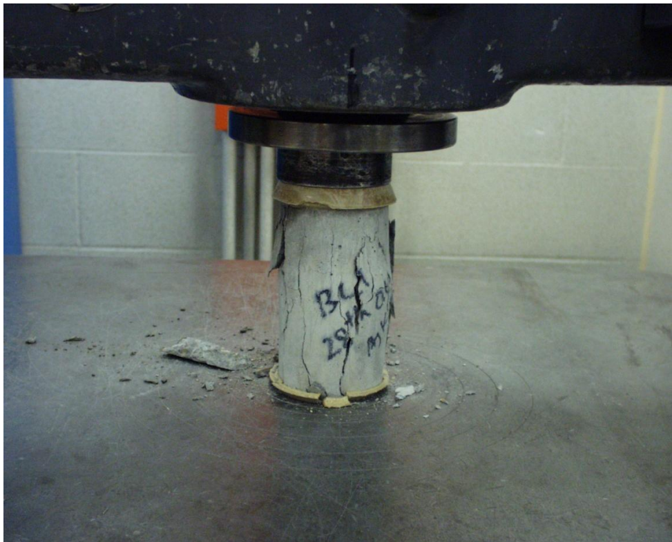
Figure 3-1: Concrete compressive test setup.
