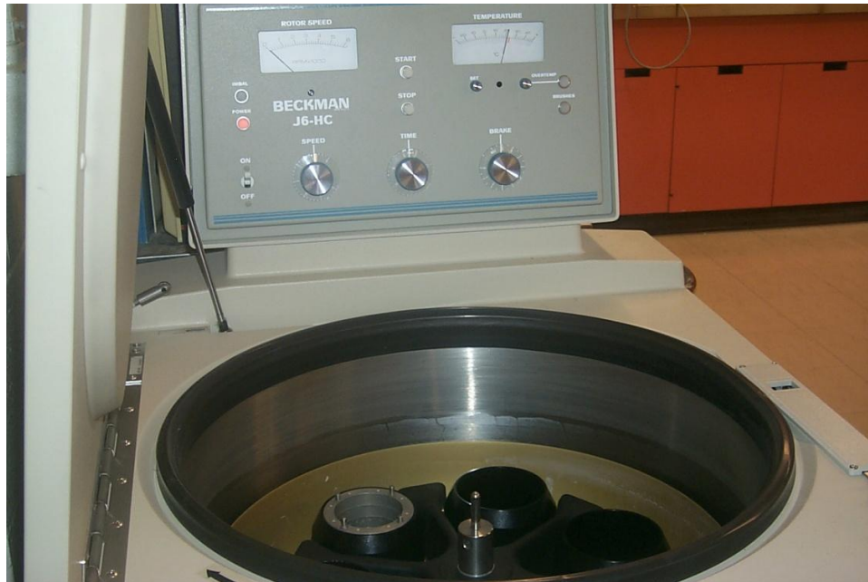
Figure 3-3: Centrifuge rotor assembly with six swinging type buckets.
