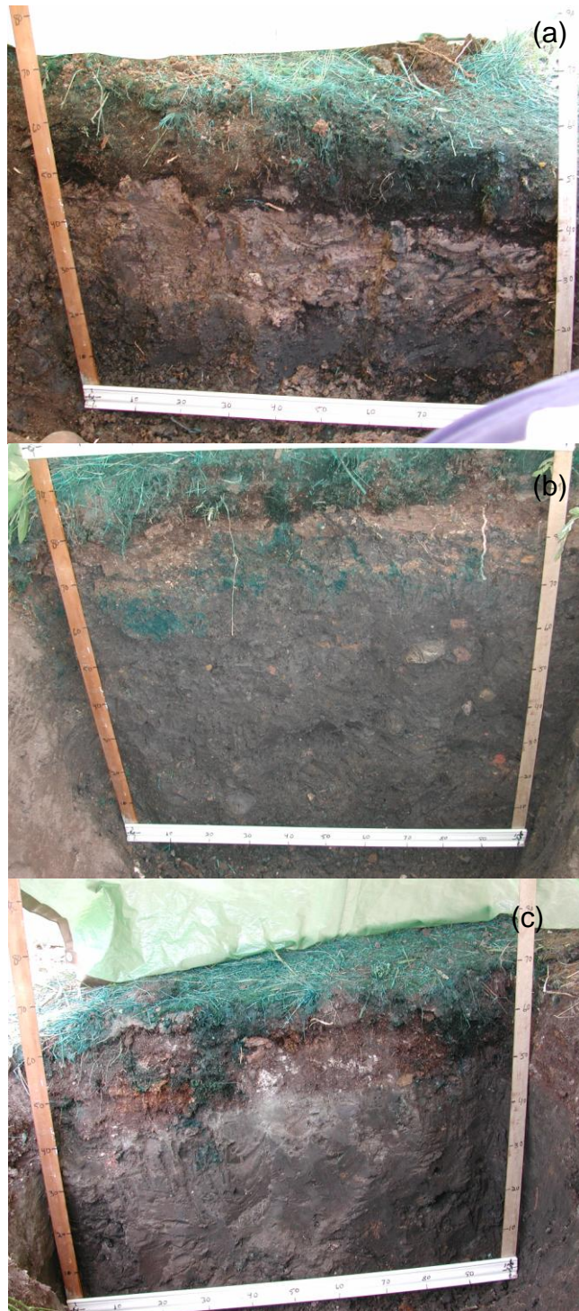
Figure 3.4 Vertical flow patterns of Brilliant Blue dye one day after soil plots were irrigated with a total application of 0.04 m dye solution. Profiles are presented for the: a)top, b)middle, and c)toe slope positions of the 0.35-m soil cover.
