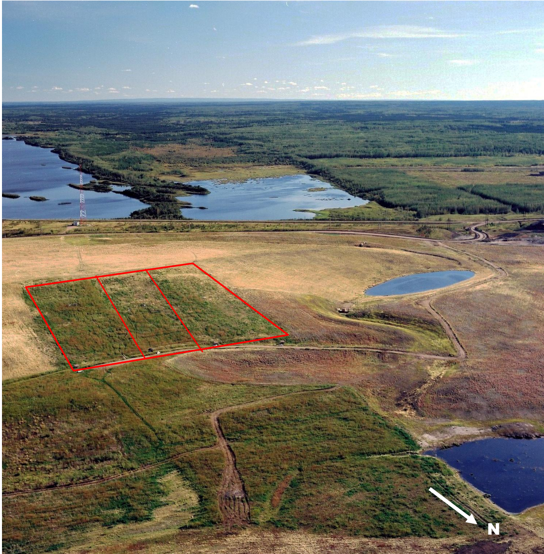
Figure 1.1 Aerial view of the South West 30 Dump (SW30) research site showing the three prototype reclamation soil covers situated along the north-facing slope (photo courtesy of Syncrude Canada Limited).
