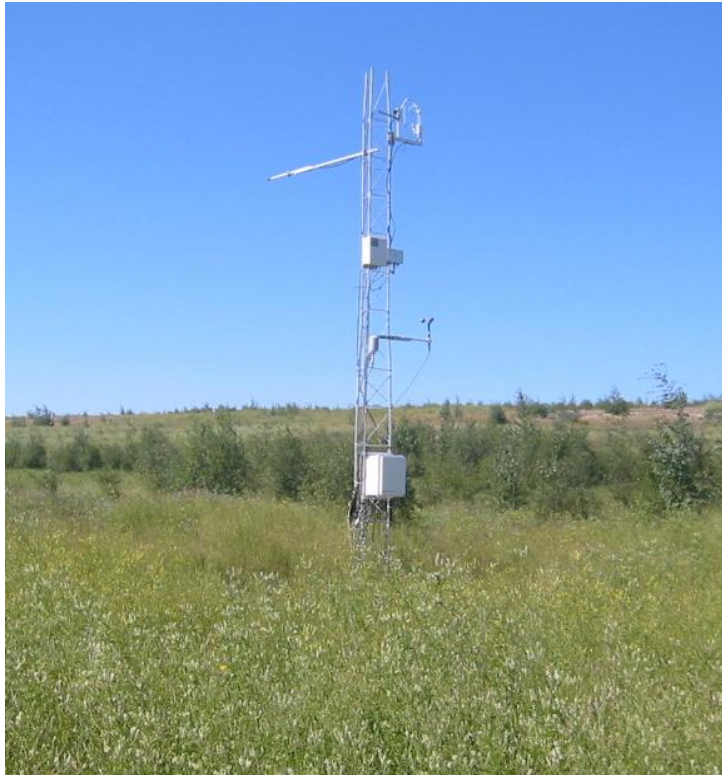
Figure 3.3. Eddy covariance tower at the SWSS site.
