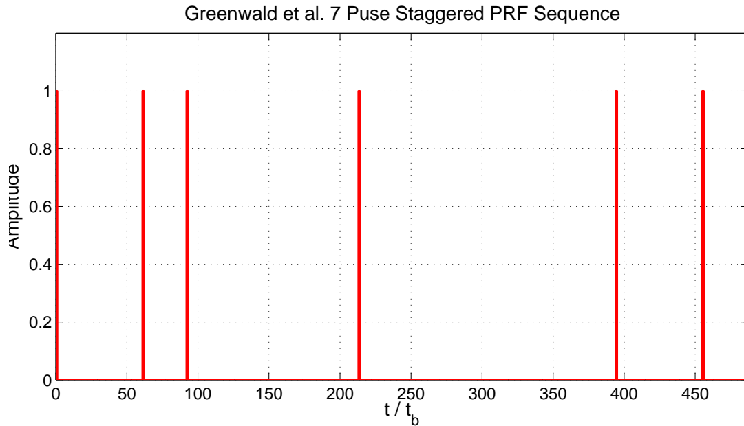
Figure 4.1: The seven-pulse staggered PRF sequence used by Greenwald et al. [1983]. The vertical axis is the amplitude of the Tx signal and the horizontal axis is the time axis in units of the waveform pulse duration t_b . In this case, T = 480t_b .
