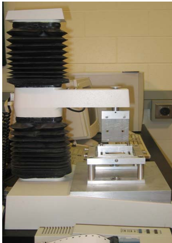
Figure 3.5. Picture of texture analyser TA.XT2.
