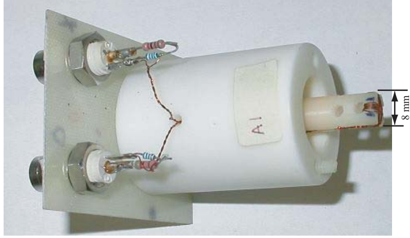
Figure 4.12: Photo of the magnetic probe in USCTI.
