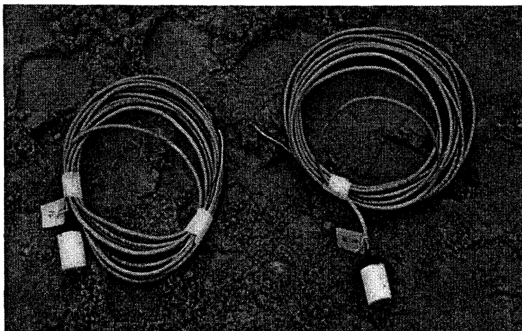
Figure 4.5 Beta-97 thermal conductivity sensors.
