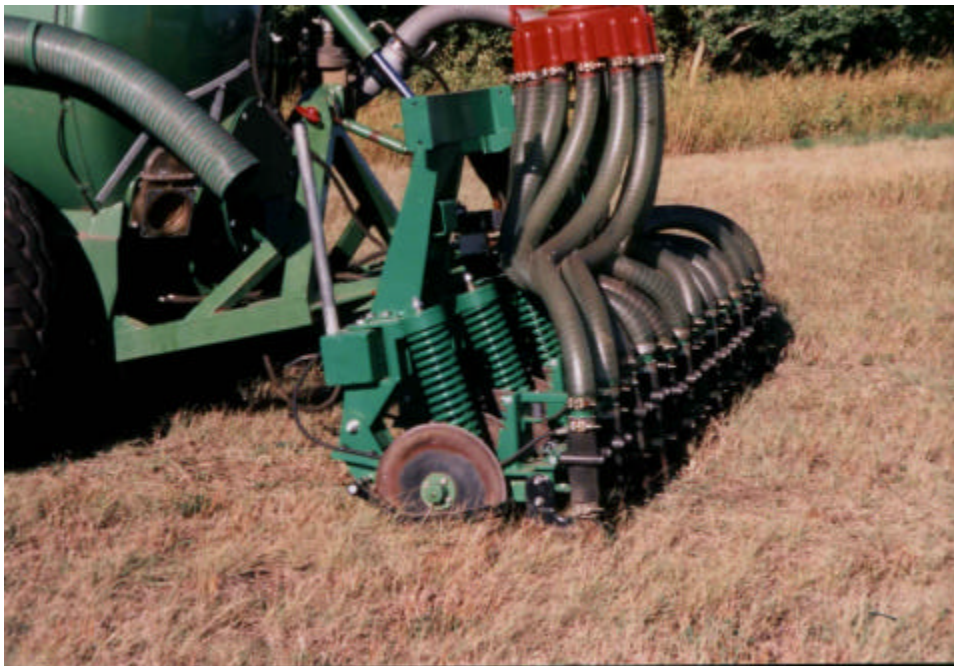
Figure 6. Greentrac Coulter/Boot System.
