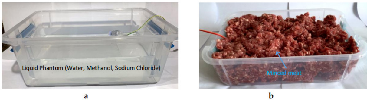
Figure 6.12 Measurement setup to test the transmission rate of the proposed capsule in: (a) liquid phantom (b) minced meat.
