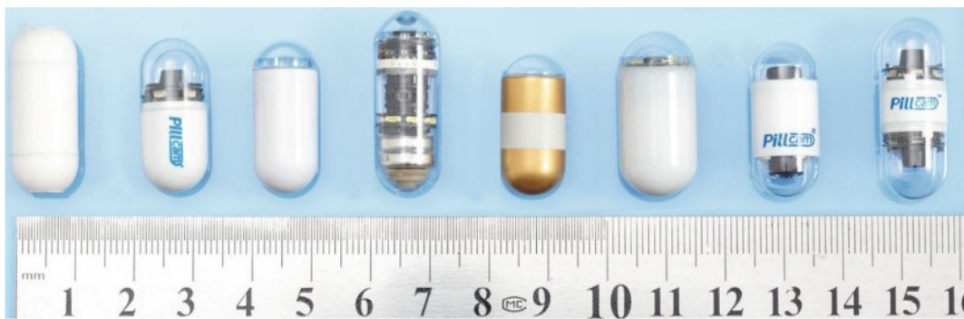
Figure 3.3 Commercial capsule endoscopes [C3.16]. Left to right: Agile patency capsule, PillCam SB2, EndoCapsule, CapsoCam, MiroCam, OMOM capsule, PillCam ESO, and PillCam COLON2.
