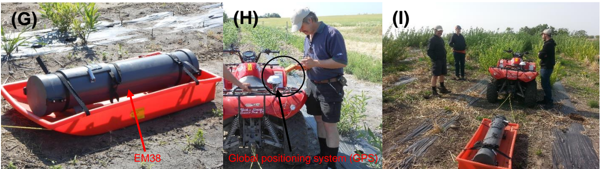
EM38 survey to measure apparent electrical conductivity of soil
