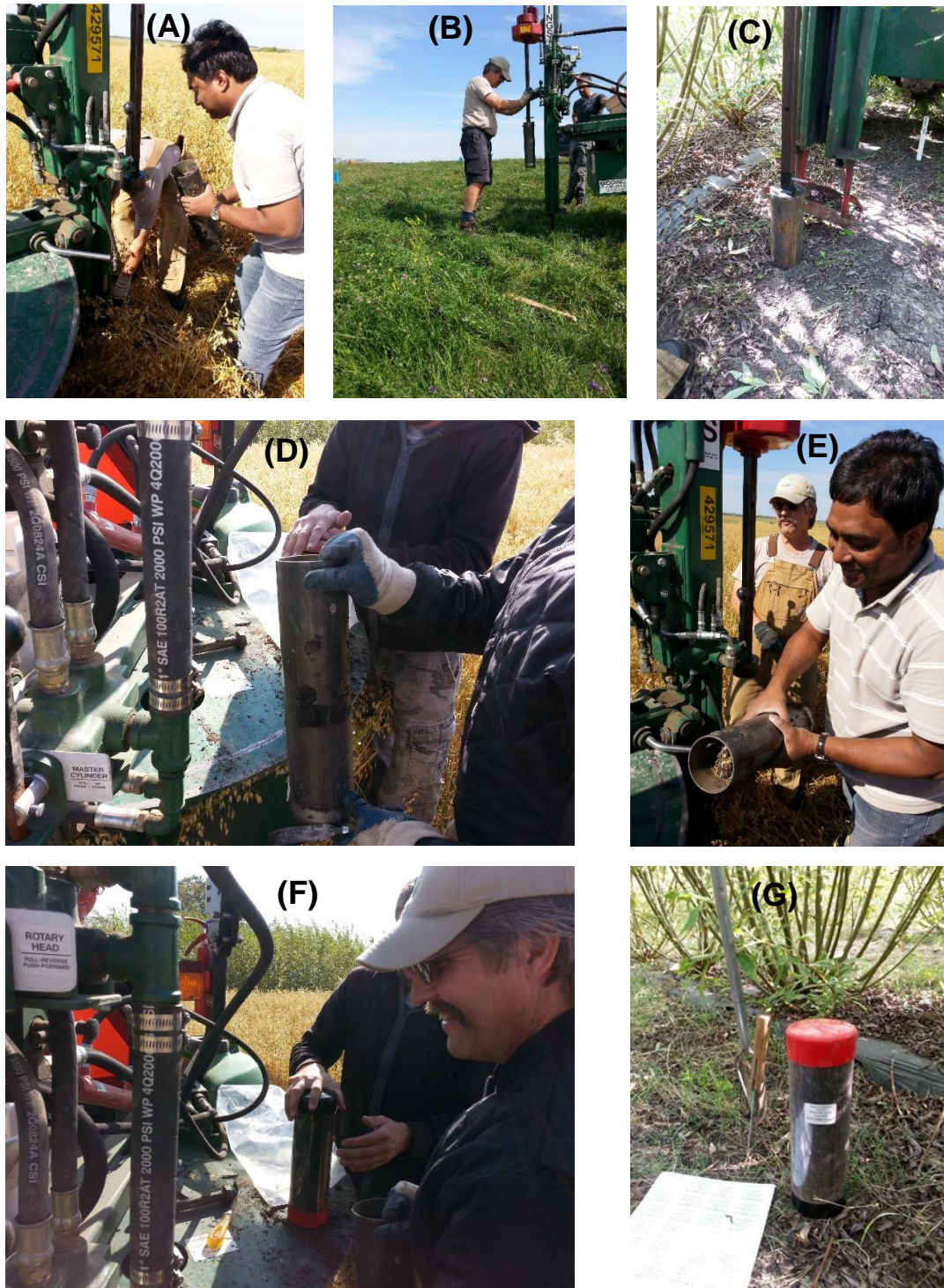
Figure D-S 9 Photographs of intact soil core samples collected from the experimental field: A) from the annual crop, B) from pasture, C) from short rotation willow, D) empty soil corer ready to mount with punch truck, E) soil corer unmounted from the punch truck after soil samples collection, F) soil core samples capped both sides and ready to transfer into the greenhouse, and G) an individual intact soil core sample.
