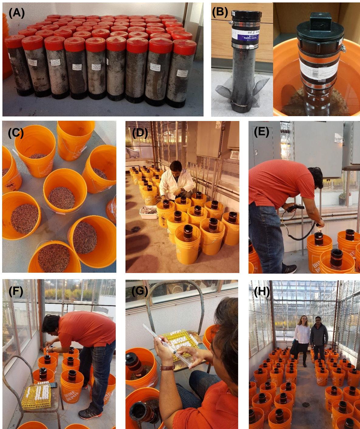
Figure D-S 10 Photographs of some activities from the microcosm incubation experiment: A) intact soil cores collected from the field, B) an individual experimental unit with and without the headspace, C) bucket filled with gravels, D) groundwater salinity measurements, E) volumetric soil water content and soil electrical conductivity measurements in the cores, F) gas samples collected from the headspaces, G) transfer of gas samples into the vials, and H) arrangement of the incubation experiment in the greenhouse.
