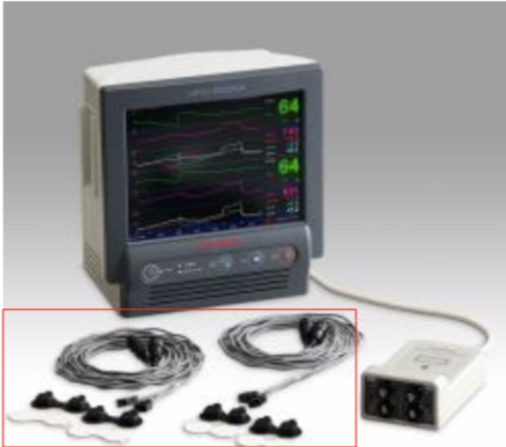
Figure 4: The NIRO-200X manufactured by Hamatsu Photonics. The light emitting and detecting electrodes have been highlighted. This is the NIRS equipment used in detecting muscle oxygenation (Hamamatsu Photonics K. K., 2018).
