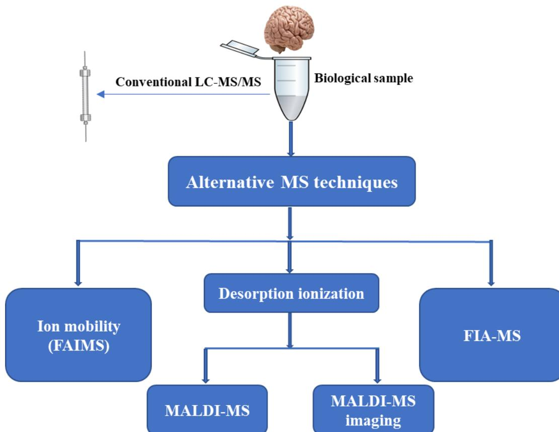
**Figure 1.** The main analytical capabilities of MS as a quantitative tool without chromatographic separation. Though not shown in the figure, high resolution instruments will enhance selectivity in quantitative assays.
