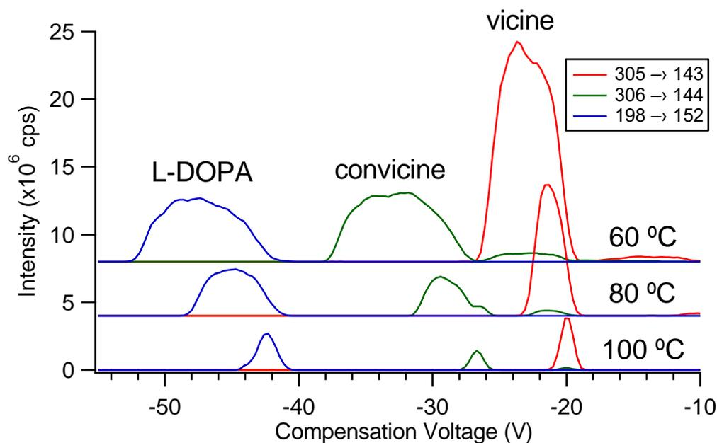
**Figure 4.** Adjusting peak separation of vicine and convicine by changing inner electrode temperature (and E/N) in FAIMS. A temperature of 60 °C was chosen for the analysis since this gives maximal signal intensity with sufficient peak separation.
