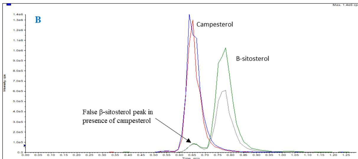
**Figure 2. A)** Interference from campesterol shows a false  $\beta$ -sitosterol peak and would be indistinguishable from the real peak due to co-elution in case of FIA-MS/MS. **B)** Fast chromatography-MS/MS showed successful separation and the false peak is distinguishable from  $\beta$ -sitosterol peak.
