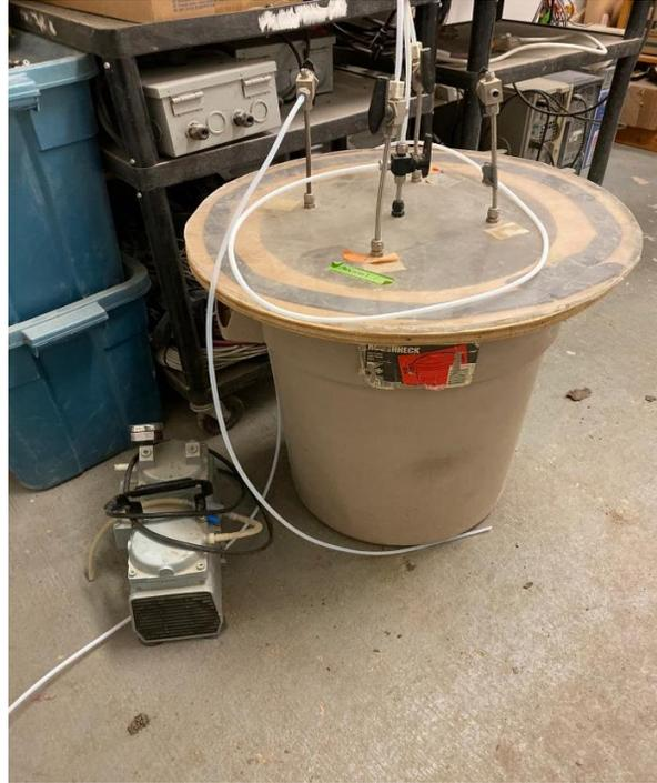
**Figure 5.2** Vacuum sampling apparatus
