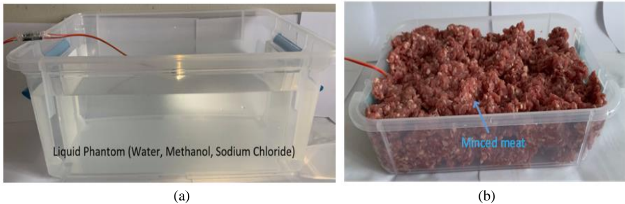
Figure 3.12 Experimental setup to test the transmission rate of the capsule in (a) liquid phantom and (b) minced meat
