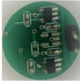
Figure 5.8 Power supply unit
