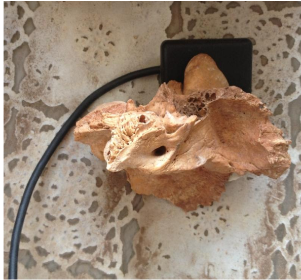
Figure 3.5: How the sensor was attached to a mastoid using modelling clay when the temporal bone was disarticulated from the rest of the cranium.
