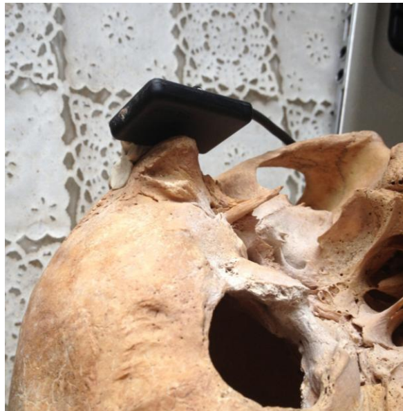
Figure 3.4: How the sensor was attached to the lateral surface of a mastoid using modelling clay.
