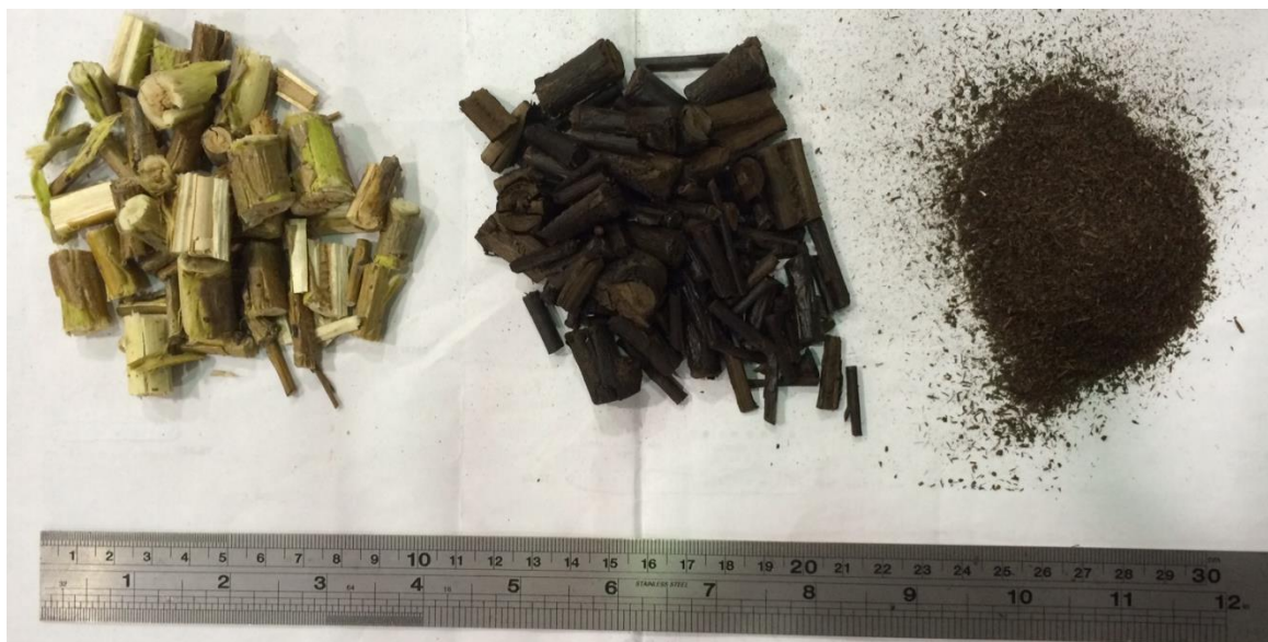
Figure 3.2: (Left to right) Non-torrefied willow segments, torrefied willow segments, and ground and torrefied willow. Segments are approximately 25 mm long and ground willow has a maximum dimension of less than 2 mm
