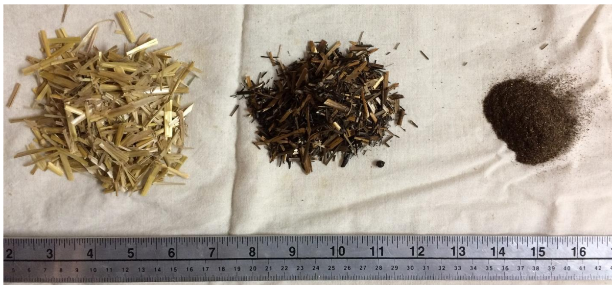
Figure 3.1: (Left to right) Non-torrefied wheat straw segments, torrefied wheat straw segments, and ground and torrefied wheat straw. Segments are 15 - 25 mm long and ground wheat straw has a maximum dimension of less than 2 mm.
