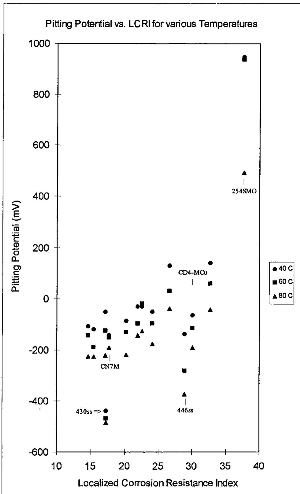
Figure 5.2 Master Plot of All Alloys Examined
