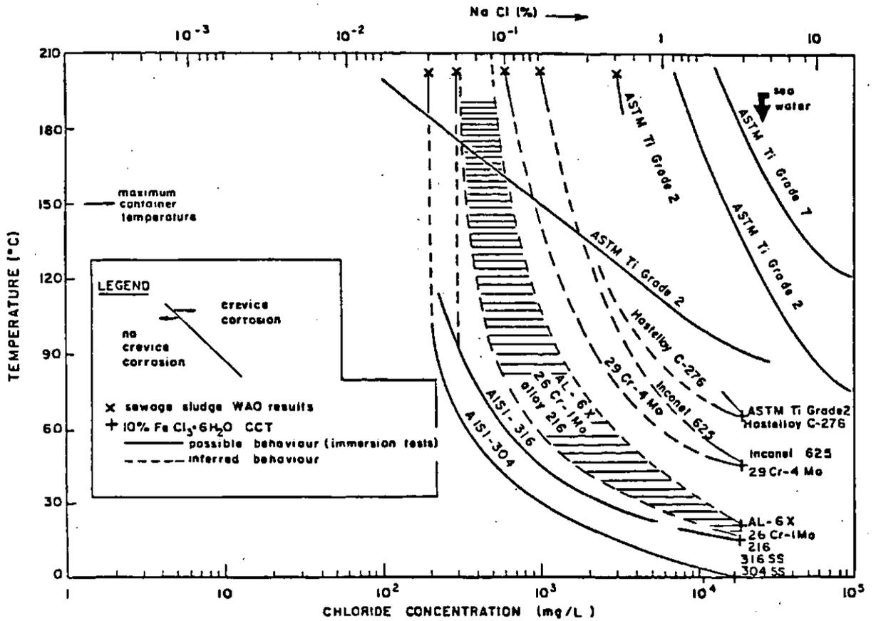
Figure 2.3 Critical Crevice Temperatures for Various Alloys in Chloride Solution
