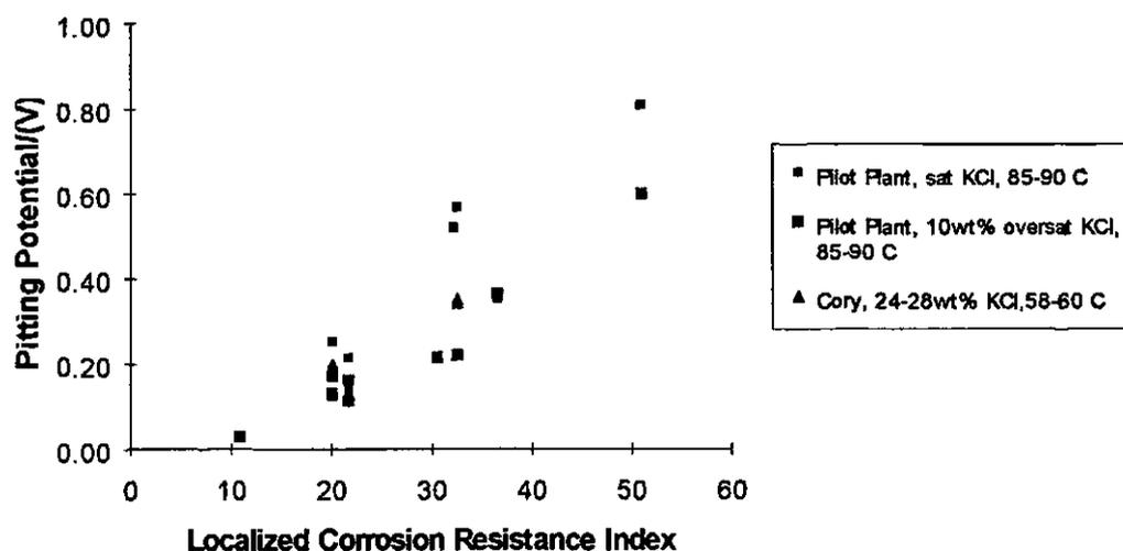
Figure 5.6 Pitting Potential (Compared to 316L Stainless Steel Eref) vs. Localized Corrosion Resistance Index
