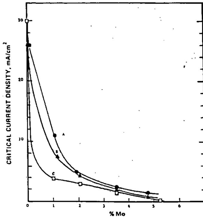
Figure 2.2 Critical Current Density vs. Molybdenum Content
