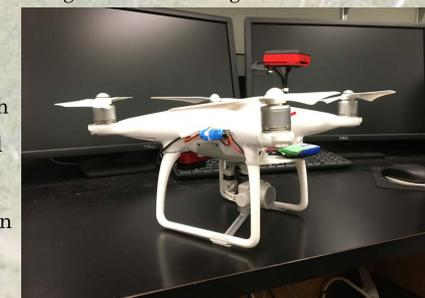
Figure 7: DJI Phantom 4 with Sequoia multispectral addition
