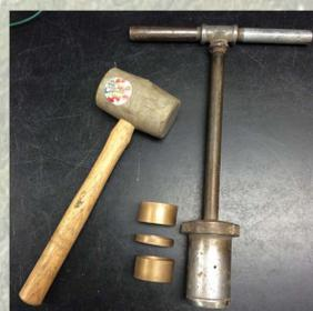
Figure 2: Vertical bulk density core sampler
