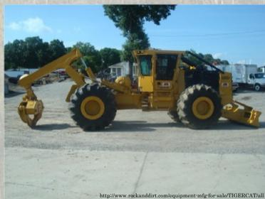
Figure 1: Skidder used to collect logs after cutting
