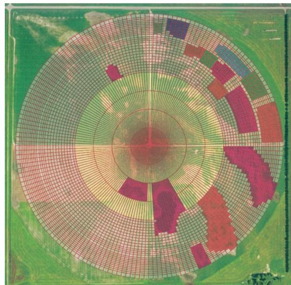
Figure 2. Diagram showing 5400 irrigation management zones in a field with VRI, and a prescription to vary irrigation amounts in areas of special soil types and research trials.
