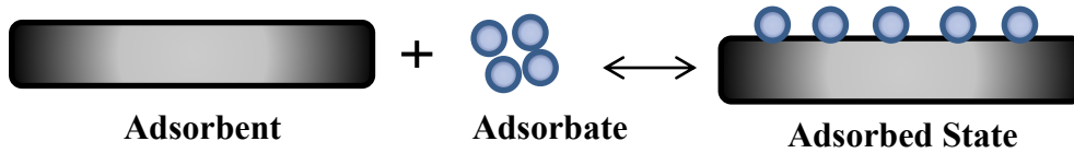
Figure 2.5 Langmuir model of gas adsorption onto a solid adsorbent.
