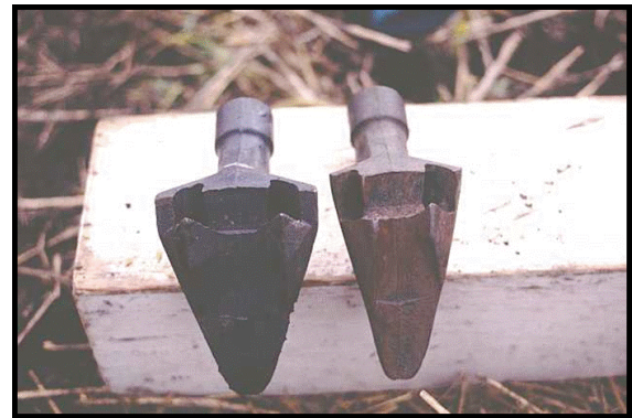
Figure 15. Worn off openers can lead to reduced separation between fertilizer and seed.
