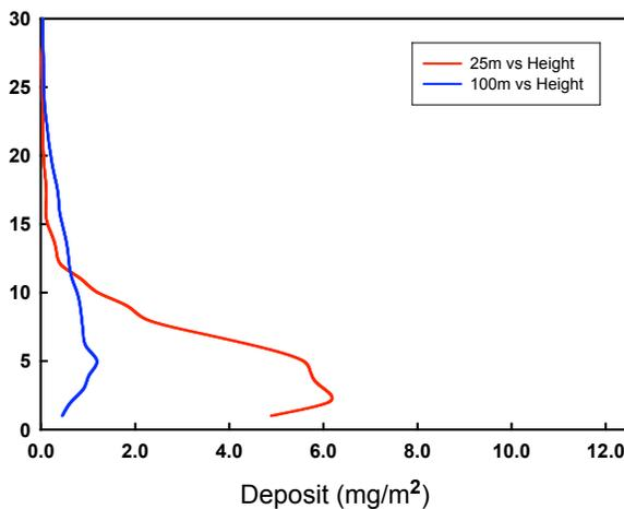
**Figure 2.** String deposit with elevation for the CP 09 30° treatment
