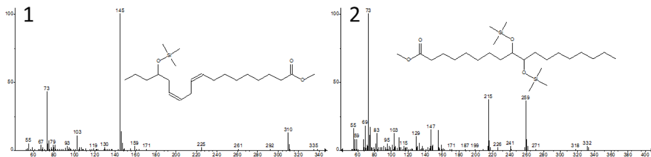
Figure 15. Mass spectra of the peaks 1 and 2 from Figure 13B. Peak 1 was identified as the TMS-derivatized FAME of 15HFA, and Peak 2 as the TMS-derivatized FAME of 9,10 dihydroxy octadecanoic acid (probably derived from hydration of 9,10-epoxy-18:0).
