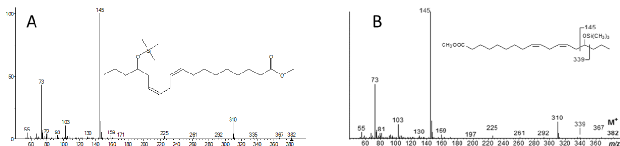
Figure 10. Mass spectrum and predicted structure of the TMS-derivatized putative 15HFA FAME. Spectrum of the peak marked with an asterisk in Figure 8B, compared to the published spectrum of the same derivatized HFA (American Oil Chemists' Society, 2012).
