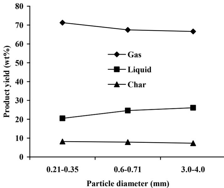
Figure 4.8 Effect of particle diameter of quartz particles on the product yield for glycerol pyrolysis at 800°C, 70mm bed height, 50mL/min of N<sub>2</sub> flow and glycerol flow rate of 5.4 g/h.
