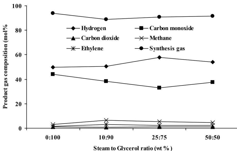
**Figure 4.21 Effect of steam on the product gas composition of glycerol gasification using silicon carbide of diameter 0.15mm as a packing material at 800°C, 70mm bed height and glycerol flow rate of 5.4 g/h.**
