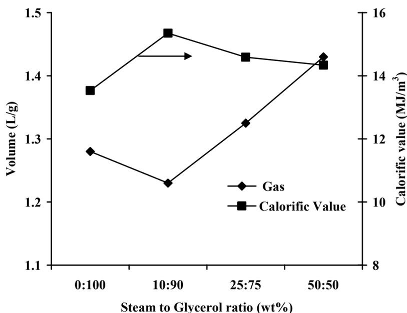
**Figure 4.22** Effects of steam on the volume and calorific value of gas during glycerol gasification using silicon carbide of diameter 0.15mm as a packing material at 800°C, 70mm bed height and glycerol flow rate of 5.4 g/h.
