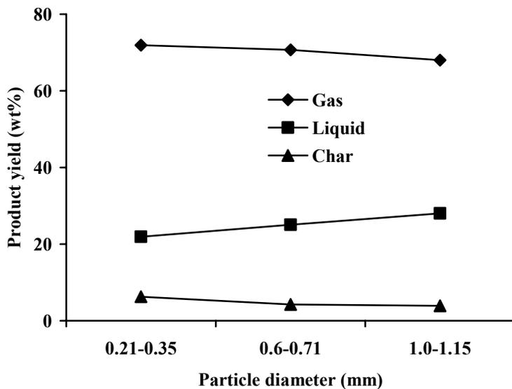
Figure 4.14 Effect of particle diameter of sand on the product yield of glycerol pyrolysis at 800°C, 70mm bed height, 50mL/min of N<sub>2</sub> flow and glycerol flow rate of 5.4 g/h.
