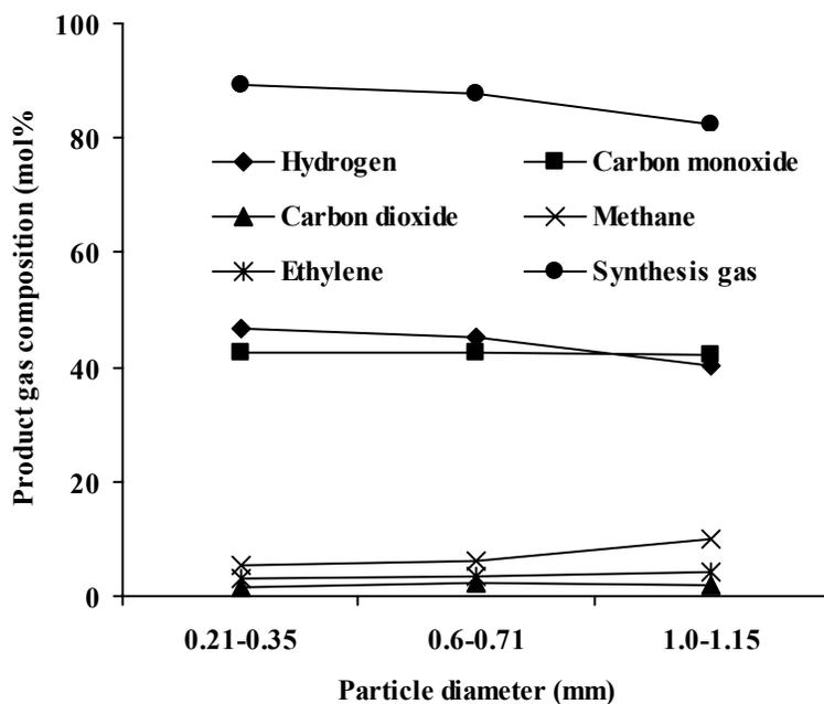
**Figure 4.15 Effect of particle diameter of sand on the product gas composition for glycerol pyrolysis at 800°C, 70mm bed height, 50mL/min of N<sub>2</sub> flow and glycerol flow rate of 5.4 g/h.**
