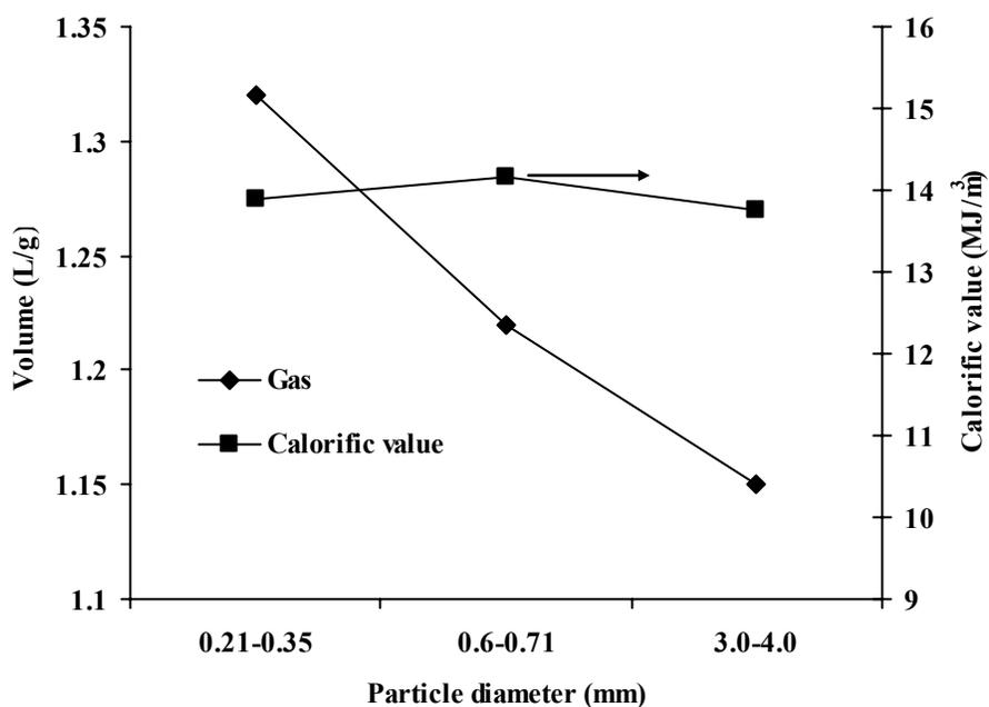
Figure 4.10 Effects of particle diameter of quartz particles on the volume and calorific value of gas for glycerol pyrolysis at 800°C, 70mm bed height, 50mL/min of N<sub>2</sub> flow and glycerol flow rate of 5.4 g/h.
