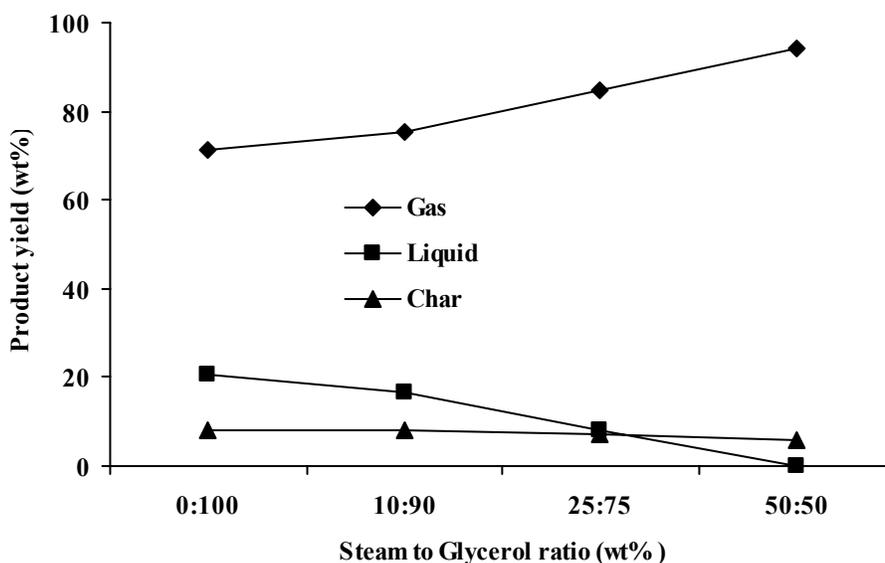
Figure 4.17 Effect of steam on the product yield of glycerol gasification using quartz of diameter 0.21-0.35mm as a packing material at 800°C, 70mm bed height and glycerol flow rate of 5.4 g/h.
