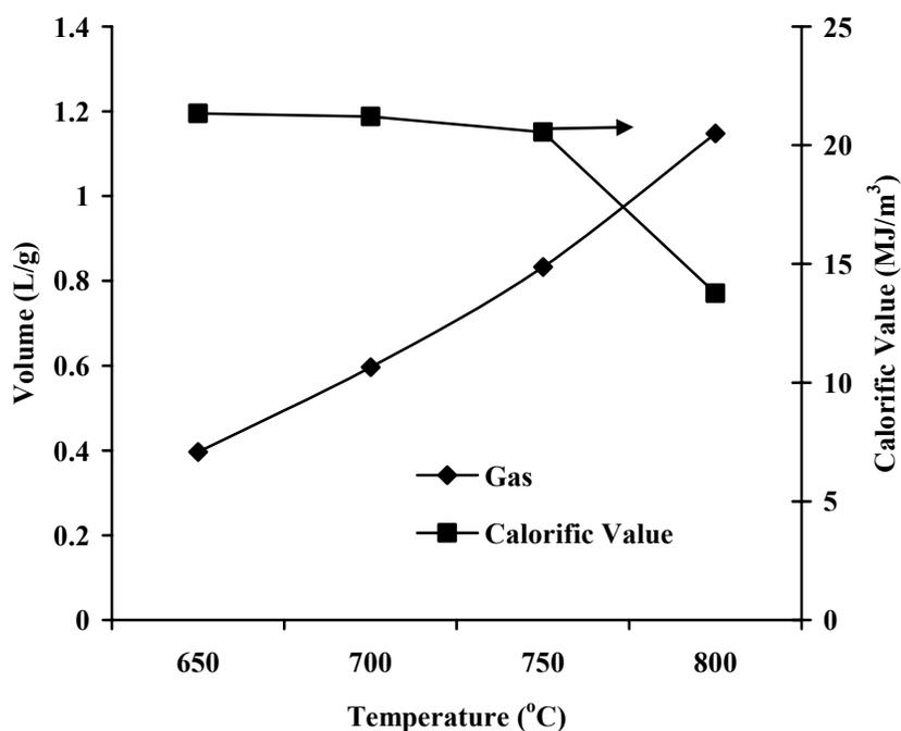
**Figure 4.7** Effects of temperature on volume and calorific value of gas during pyrolysis of glycerol at carrier gas flow rate 50mL/min, 70mm bed height, quartz particle of diameter 3-4mm and glycerol flow rate 5.4g/h.
