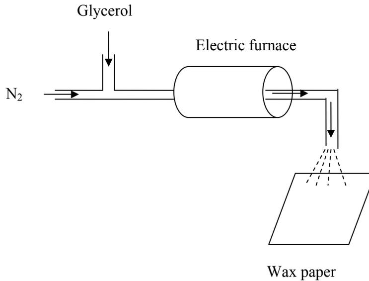
**Figure 3.1: Set up for the spray studies**
