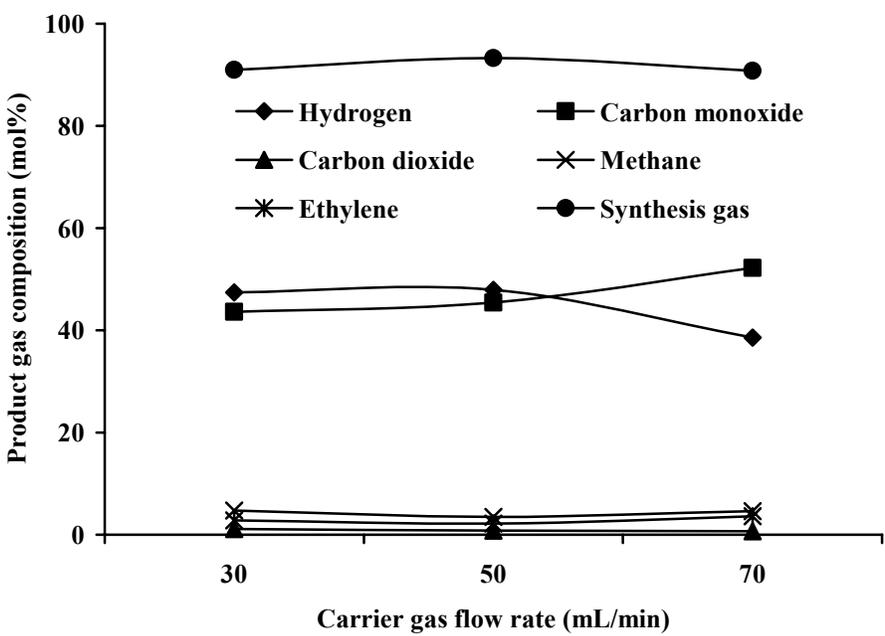
Figure 4.3 Effect of carrier gas flow (N<sub>2</sub>) on product composition during pyrolysis of glycerol at 800°C, 70mm bed height and glycerol flow rate 5.4g/h.
