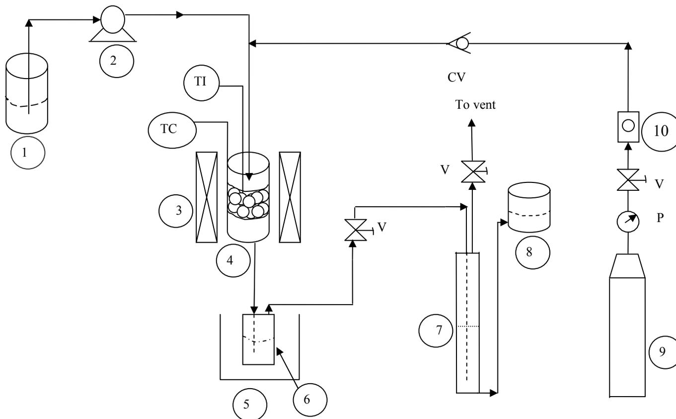
**Figure 3.2 Experimental set up for pyrolysis of glycerol.**
