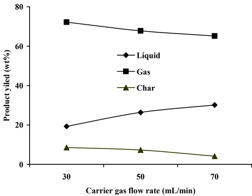
Figure 4.2 Effect of carrier gas flow (N<sub>2</sub>) on product yield during pyrolysis of glycerol at 800°C, bed height 70mm and glycerol flow rate 5.4 g/h.
