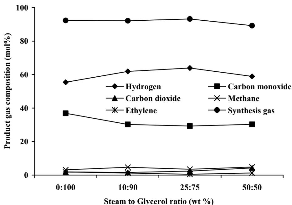
**Figure 4.18 Effect of steam on the product gas composition of glycerol gasification using quartz of diameter 0.21-0.35mm as a packing material at 800°C, 70mm bed height and glycerol flow rate of 5.4 g/h.**
