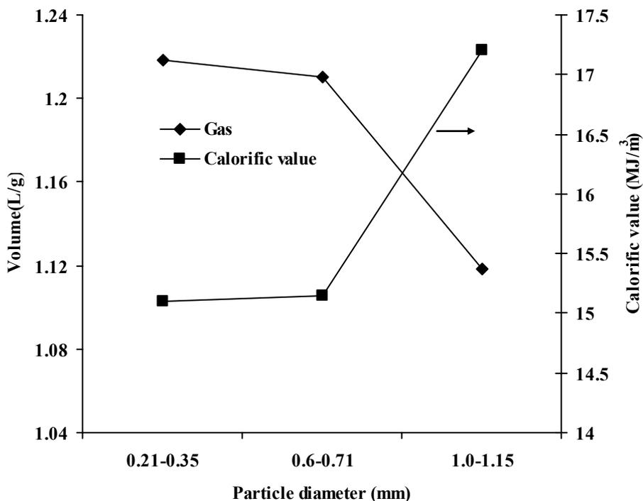
**Figure 4.16** Effects of particle diameter of sand on volume and calorific value of gas for glycerol pyrolysis at 800°C, 70mm bed height, 50mL/min of N<sub>2</sub> flow and glycerol flow rate of 5.4 g/h.
