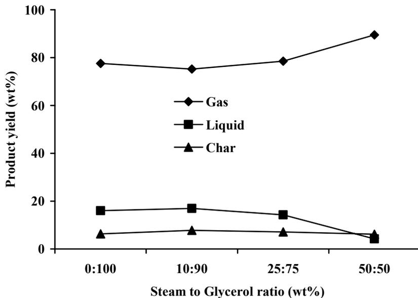
**Figure 4.20 Effect of steam on the product yield of glycerol gasification using silicon carbide of diameter 0.15mm as a packing material at 800°C, 70mm bed height and glycerol flow rate of 5.4 g/h.**
