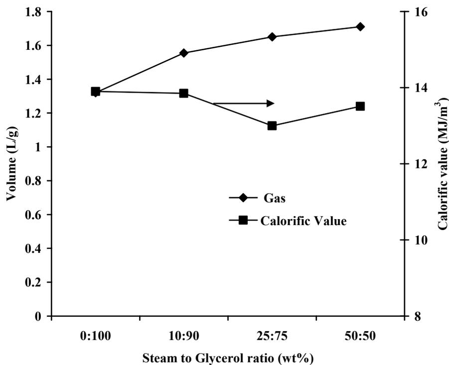
**Figure 4.19** Effects of steam on the volume and calorific value of gas during glycerol gasification using quartz of diameter 0.21-0.35mm as a packing material at 800°C, 70mm bed height and glycerol flow rate of 5.4 g/h.
