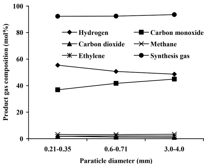
Figure 4.9 Effect of particle diameter of quartz particles on the product gas composition for glycerol pyrolysis at 800°C, 70mm bed height, 50mL/min of N<sub>2</sub> flow and glycerol flow rate of 5.4 g/h.
