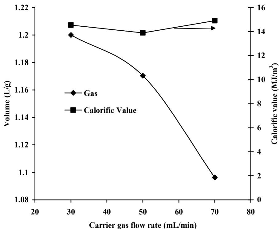
**Figure 4.4 Effects of carrier gas flow (N<sub>2</sub>) on volume and calorific value of gas during the pyrolysis at 800°C, 70mm bed height and glycerol flow rate 5.4g/h.**
