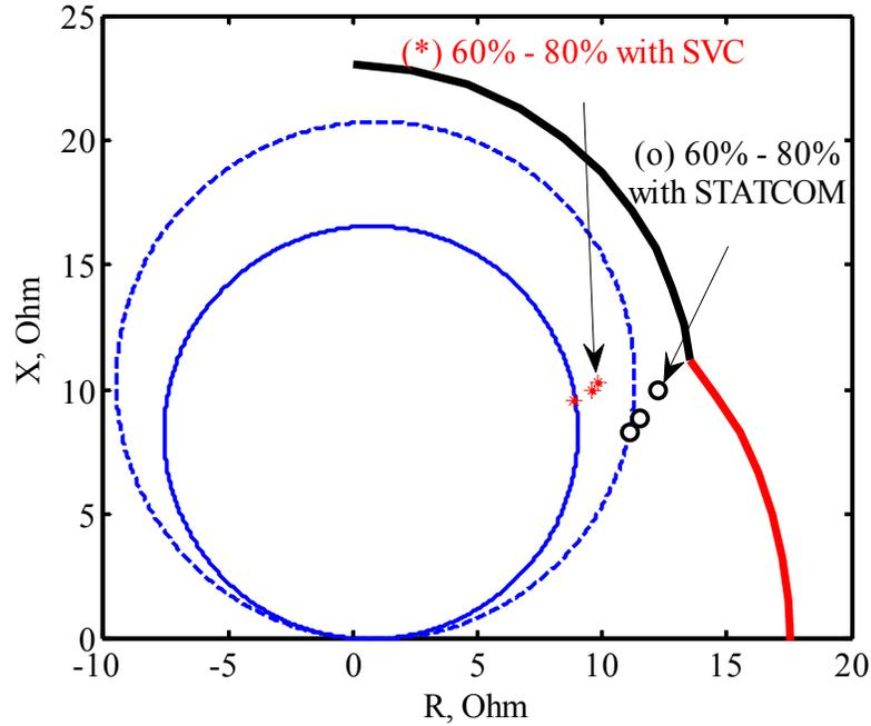
**Figure 2.33.** Impacts of the midpoint STATCOM and SVC on the coordination between Relay (21) and GOEC limit for three-phase faults on Line 1 in System II at the relay reach (the percentages are the generator loading).
