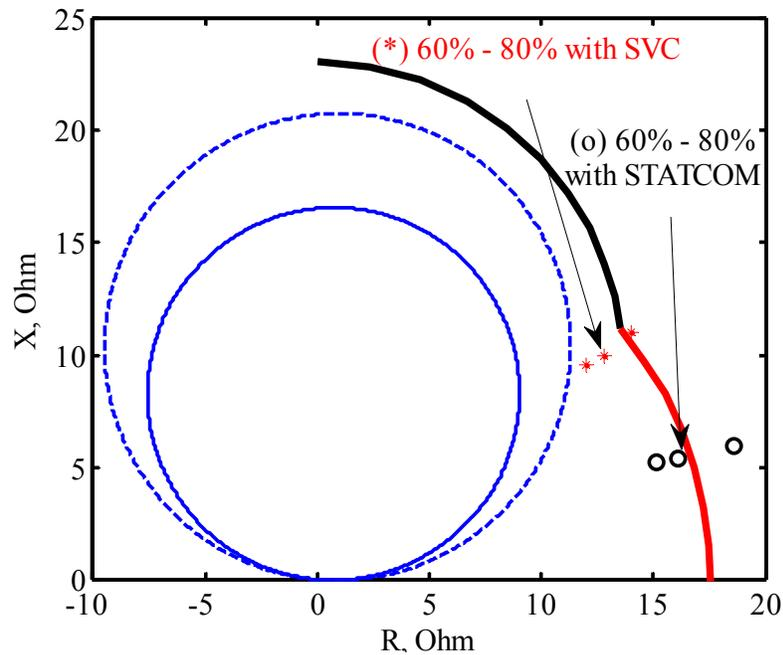
**Figure 2.34.** Impacts of the midpoint STATCOM and SVC on the coordination between Relay (21) and GOEC limit for line-to-line faults on Line 1 in System II at the relay reach (the percentages are the generator loading).
