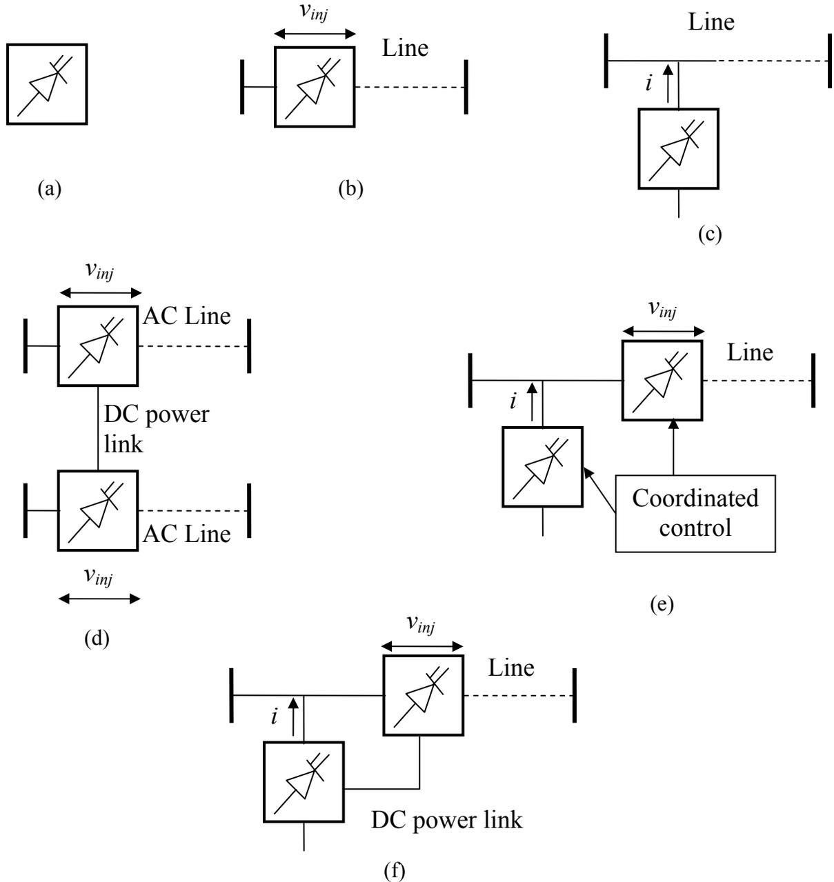
**Figure 1.1.** Basic types of FACTS Controllers: (a) general symbol for a FACTS Controller, (b) series controller, (c) shunt controller, (d) unified series-series controller, (e) coordinated series and shunt controller, (f) unified series-shunt controller.
