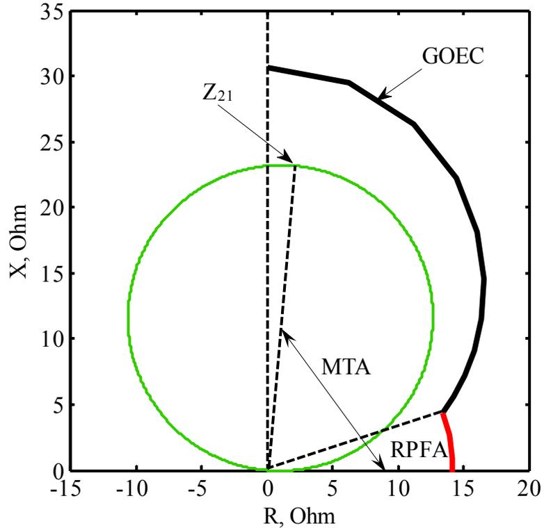
**Figure 4.3.** Coordination between Relay (21), when it is set for generator thermal backup protection and  $G_1$  steady-state overexcited capability limit (System I).
