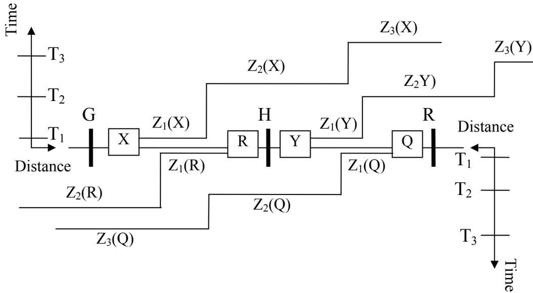
**Figure 1.4.** Zoned distance protection on adjacent transmission lines.
