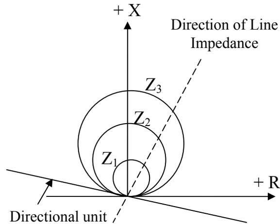
**Figure 1.3.** Distance protection zones in the Z plane.
