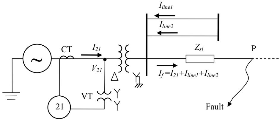
**Figure 2.17.** Apparent impedance measurement with system infeed currents.
