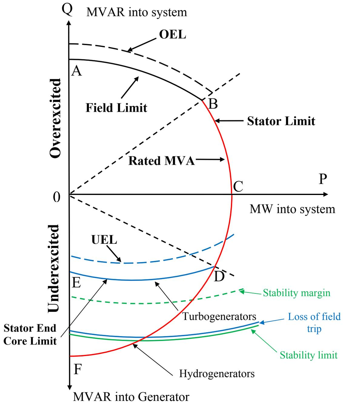
**Figure 2.9.** Generator capability curves for turbogenerators and hydrogenerators.
