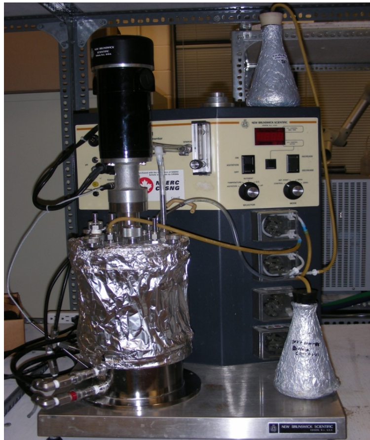
Figure 6.1 Continuous stirred tank reactor for biodegradation of 1,4-benzoquinone.
