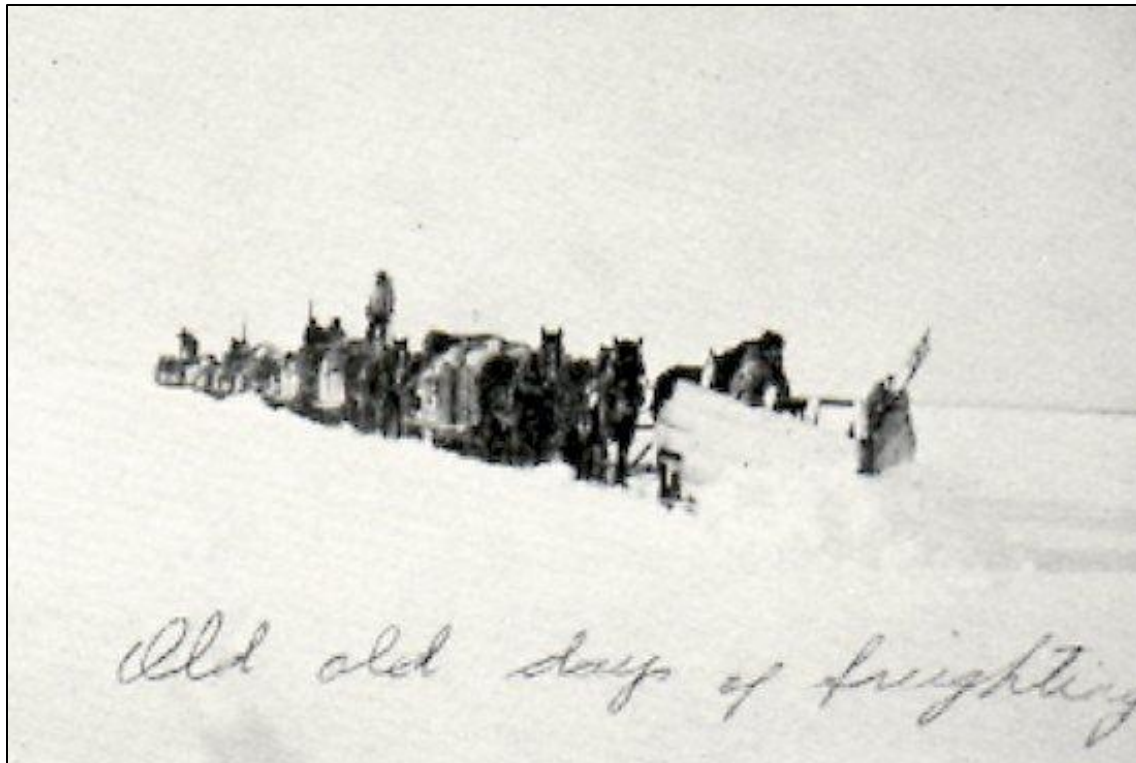
Figure 27. Crossing a northern lake in winter with a 'freight swing.' Note plow in front. www.jkcc.com .
