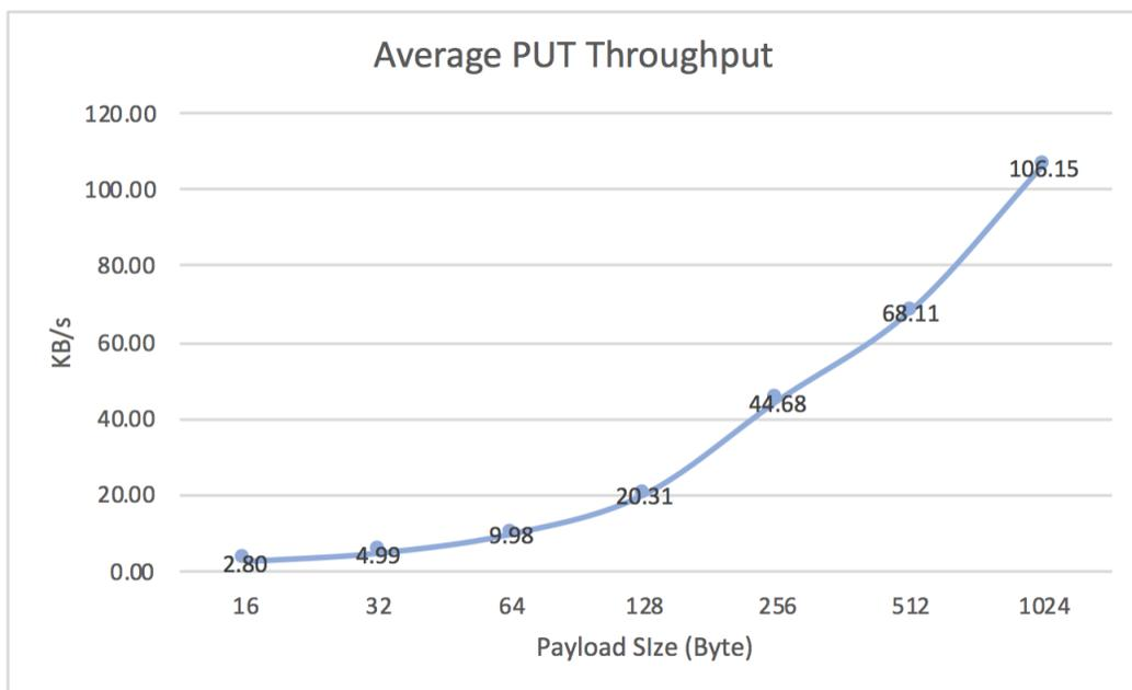
**Figure 5.13:** Average PUT Throughput for Various Payload Size
