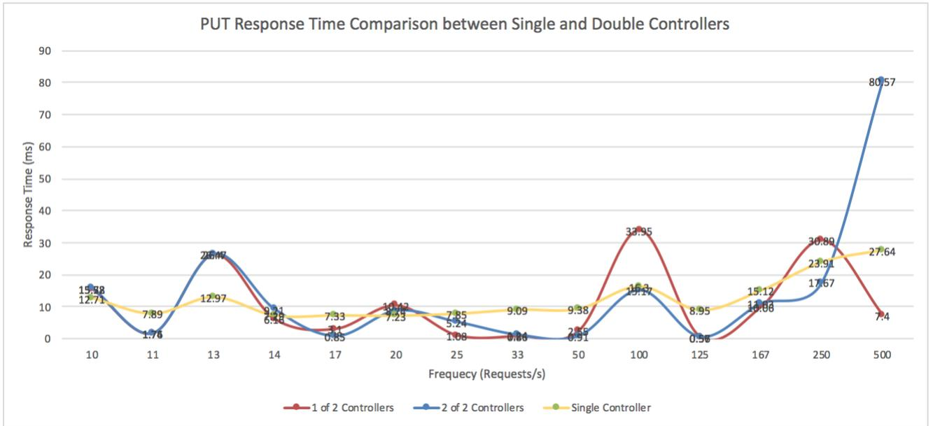
Figure 5.20: PUT Response Time Comparison between Single and Two Controllers
