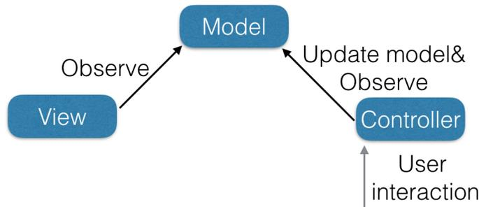
**Figure 3.1:** The Model-View-Controller pattern
