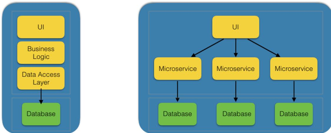
**Figure 3.5:** Monolithic Architecture and Micro-Service Architecture
