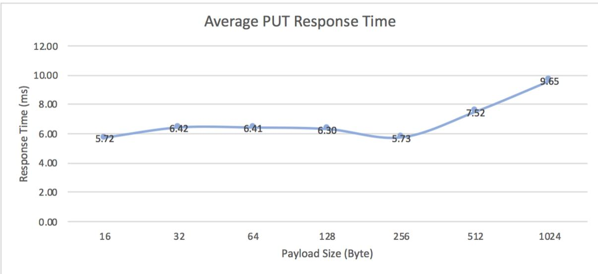
**Figure 5.11:** Average PUT Response Time for Various Payload Size
