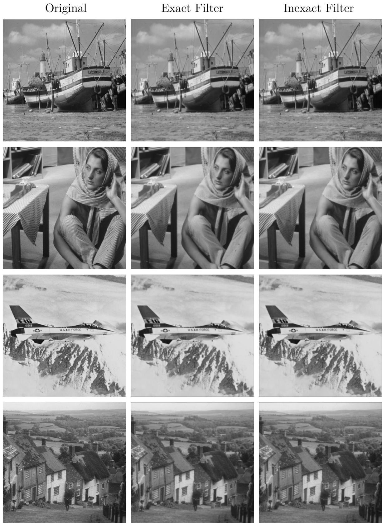
Fig. 5.9. Images used in  $7 \times 7$  Gaussian blur application from top to bottom: boat, barbara, airplane, and goldhill. The first column contains original images used as input, the second column is the result from convolution computed using exact operations, and the third column contains the outputs of the convolution computed by ABM-MAC.
