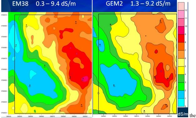
depths of 30-60 cm, the predicted EC values were closer, but the EM38 still showed a slightly wider dynamic range than the GEM2. One of the reasons for this variability between the two EM sensors might be that the sampling depths of 30 cm increments down to 1.2 m were closer to the
