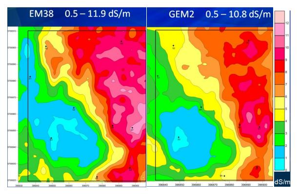
The maps of predicted EC values for the 0-30 cm depth were quite similar between the EM 38 and the GEM2, with the EM38 showing a slightly wider dynamic range than the GEM2. For
