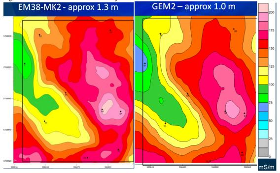
depths, the EM38 also showed slightly higher levels of conductivity, probably because it was imaging through a greater volume of soil as it was penetrating to slightly greater depth than the GEM2. The corollary of this is that the frequencies chosen for the GEM2 did appear to be reasonable approximations of the depths of penetration with respect to the EM38.
