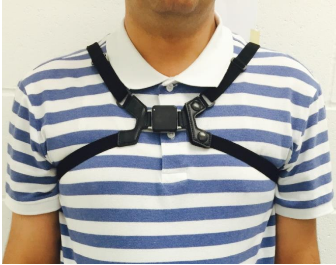
Figure 2: Inertial sensor strapped on the chest to assess trunk posture
