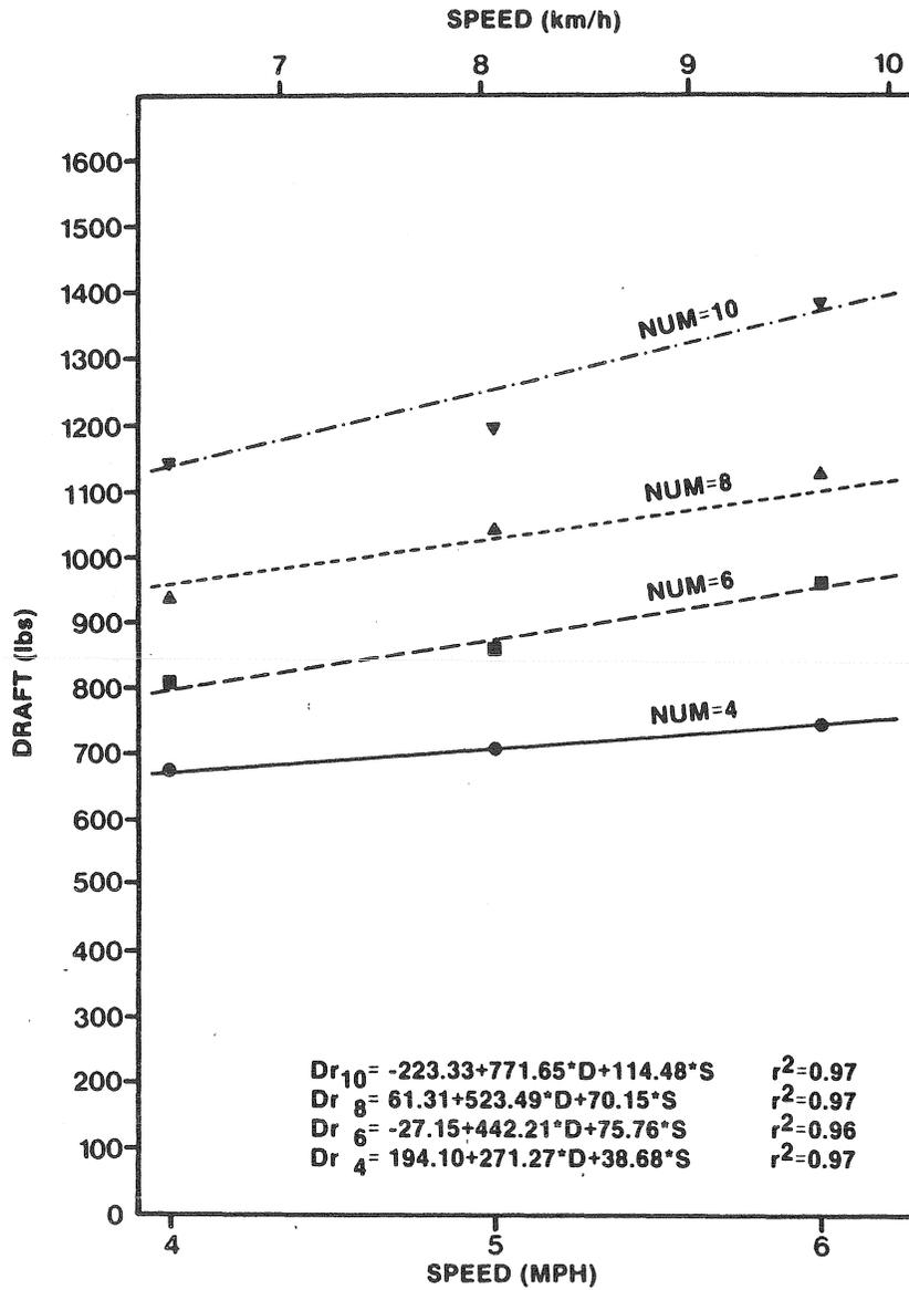
Figure 11. DRAFT VERSUS SPEED FOR FOUR, SIX, EIGHT AND TEN OPENERS, AVERAGE OF FOUR OPENER TYPES AND FIVE DEPTHS.
