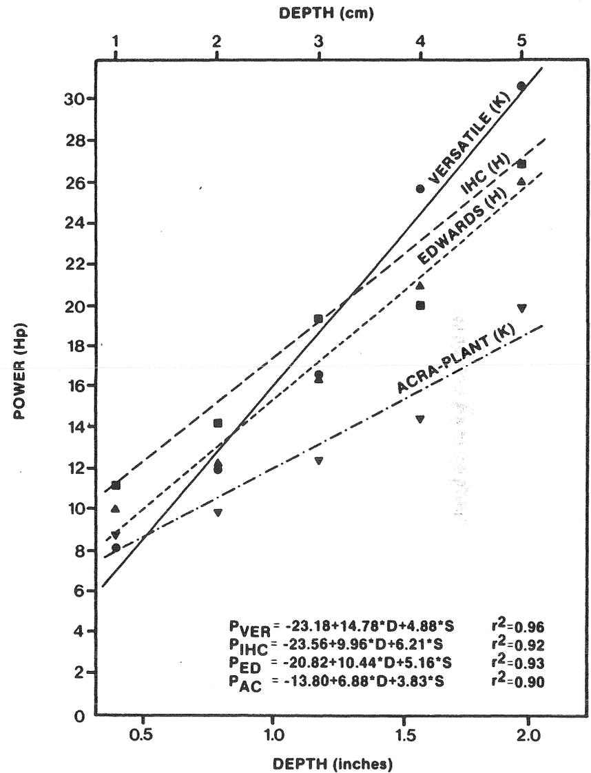
Figure 8. POWER REQUIREMENTS VERSUS SEEDING DEPTH FOR FOUR TYPES OF OPENERS. AVERAGE SPEED WITH TEN OPENERS.
