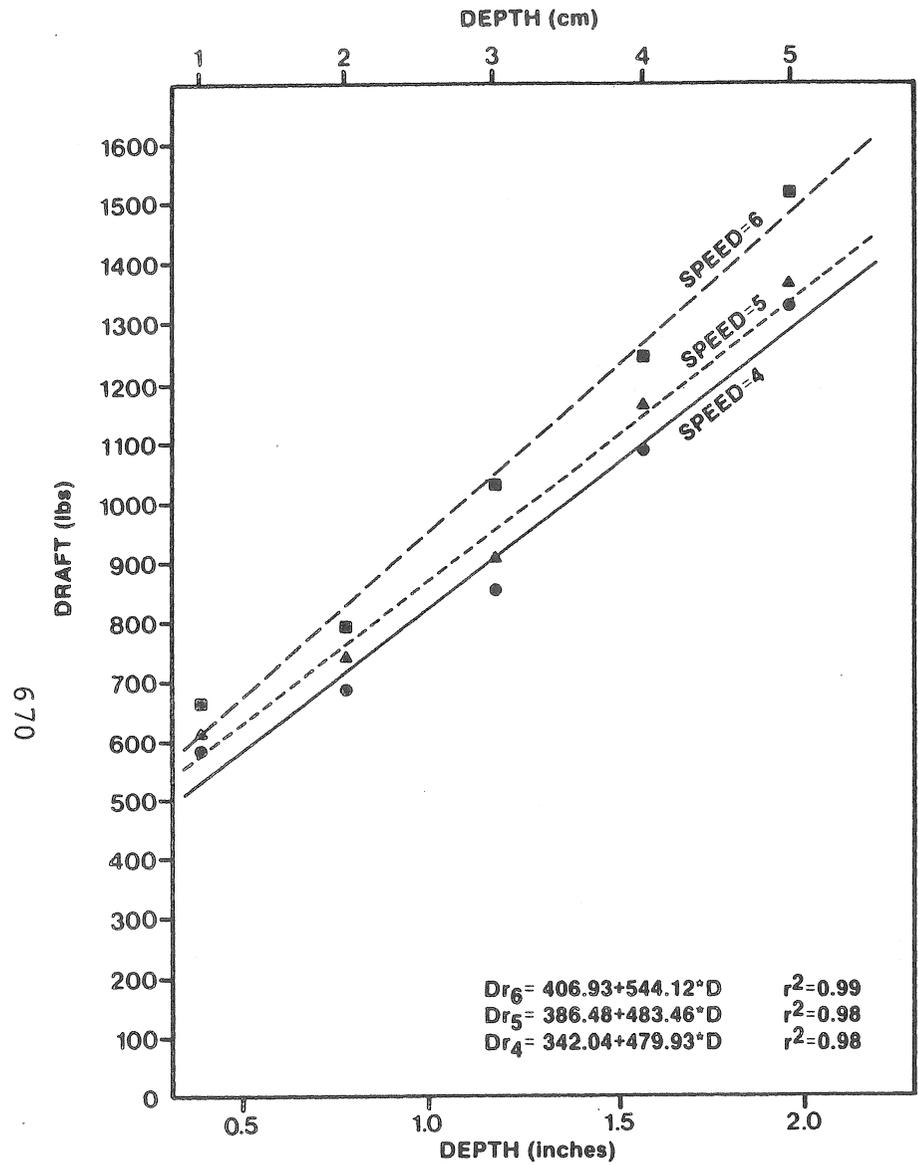
Figure 9. DRAFT VERSUS SEEDING DEPTH FOR THREE SPEEDS. AVERAGE DRAFT FOR ALL OPENER TYPES IN TRIALS WITH FOUR, SIX, EIGHT AND TEN OPENERS.
