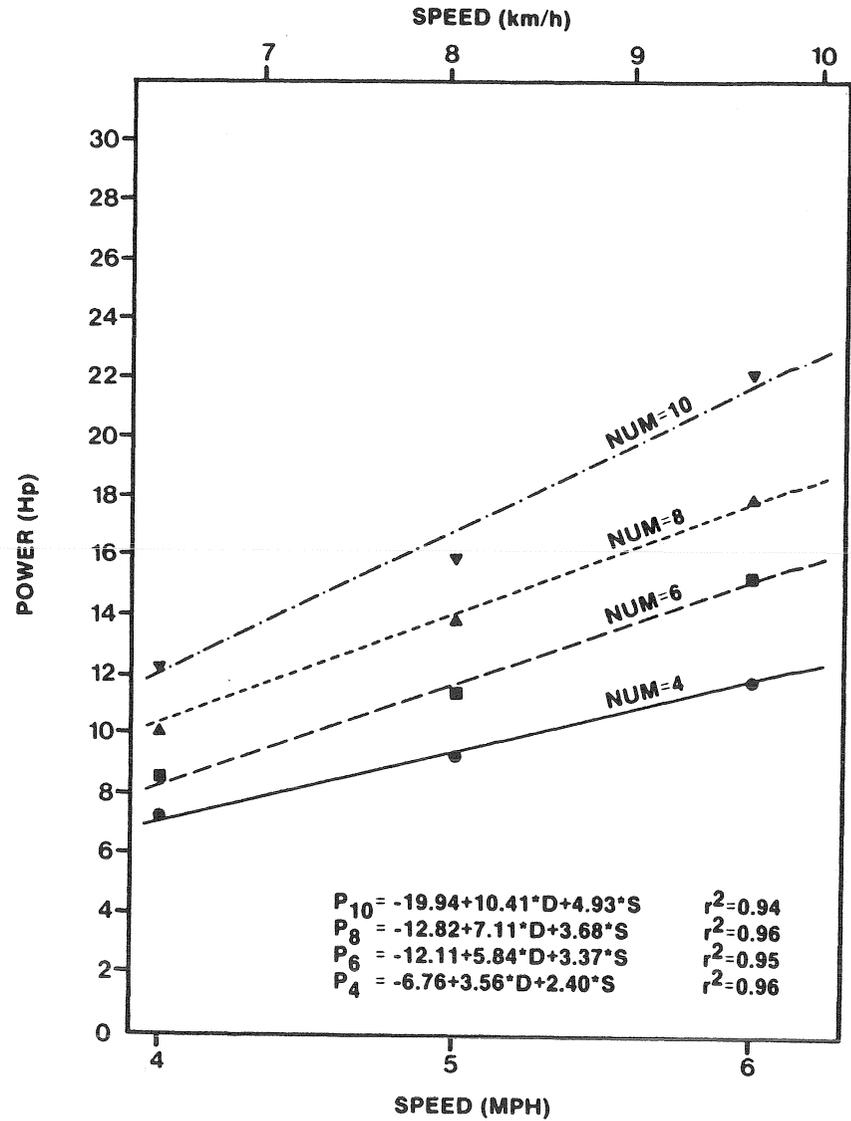
Figure 12. POWER VERSUS SPEED FOR FOUR, SIX, EIGHT AND TEN OPENERS, AVERAGE OF FOUR OPENER TYPES AND FIVE DEPTHS.
