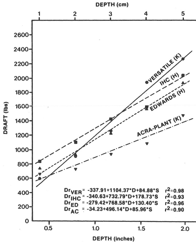
FIGURE 7. DRAFT VERSUS SEEDING DEPTH FOR FOUR TYPES OF OPENERS. AVERAGE SPEED WITH TEN OPENERS.
