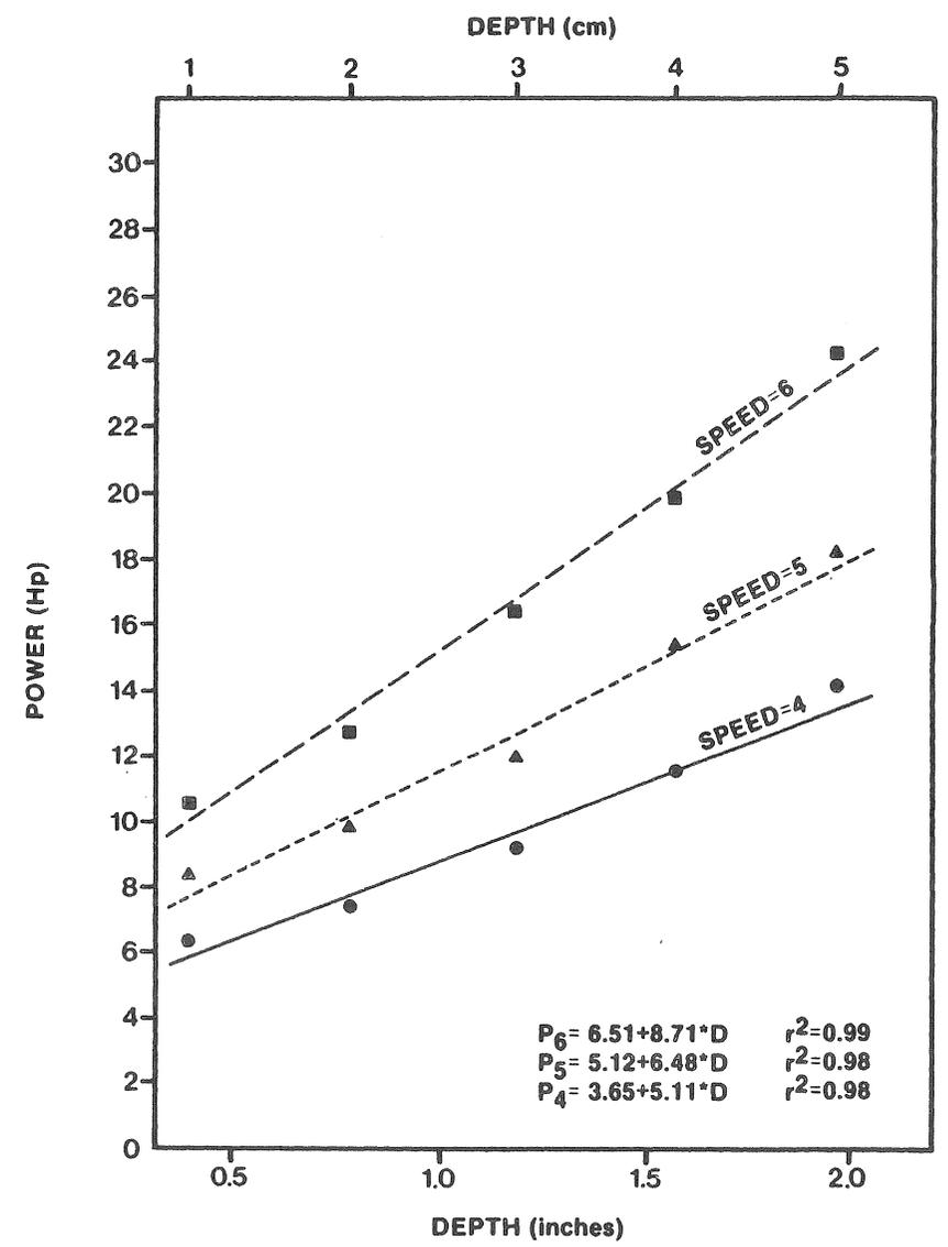
Figure 10. POWER VERSUS SEEDING DEPTH FOR THREE SPEEDS. AVERAGE POWER FOR ALL OPENER TYPES IN TRIALS WITH FOUR, SIX, EIGHT AND TEN OPENERS.
