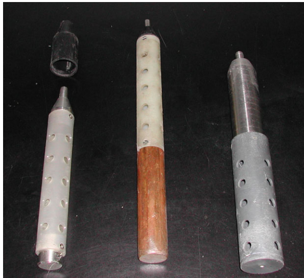
Figure 4.5 – Suction strainers used with samplers in successive redesigns (left to right).
