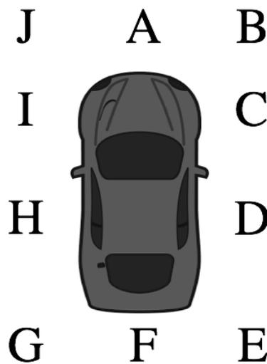
*Figure 5-1.* The subject vehicle is pictured. The position of impact is the location of the conflicting vehicle, person, animal, or object in relation to the subject vehicle. The position of impact was coded as one of ten (A-J) possible locations on the vehicle.
