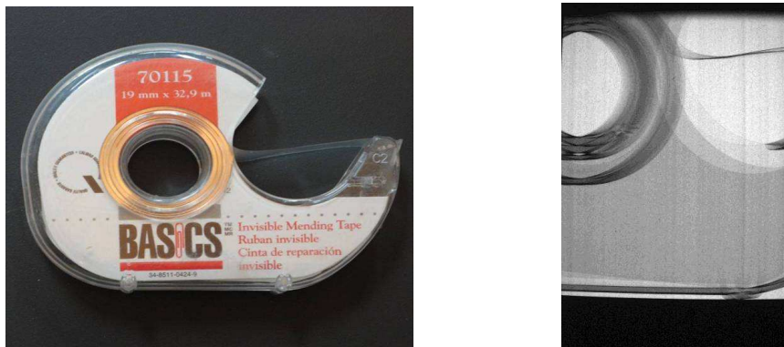
Figure 7.4: A picture of the first analyzer based imaging sample and the resulting x-ray image from the SyLMAND tests.
