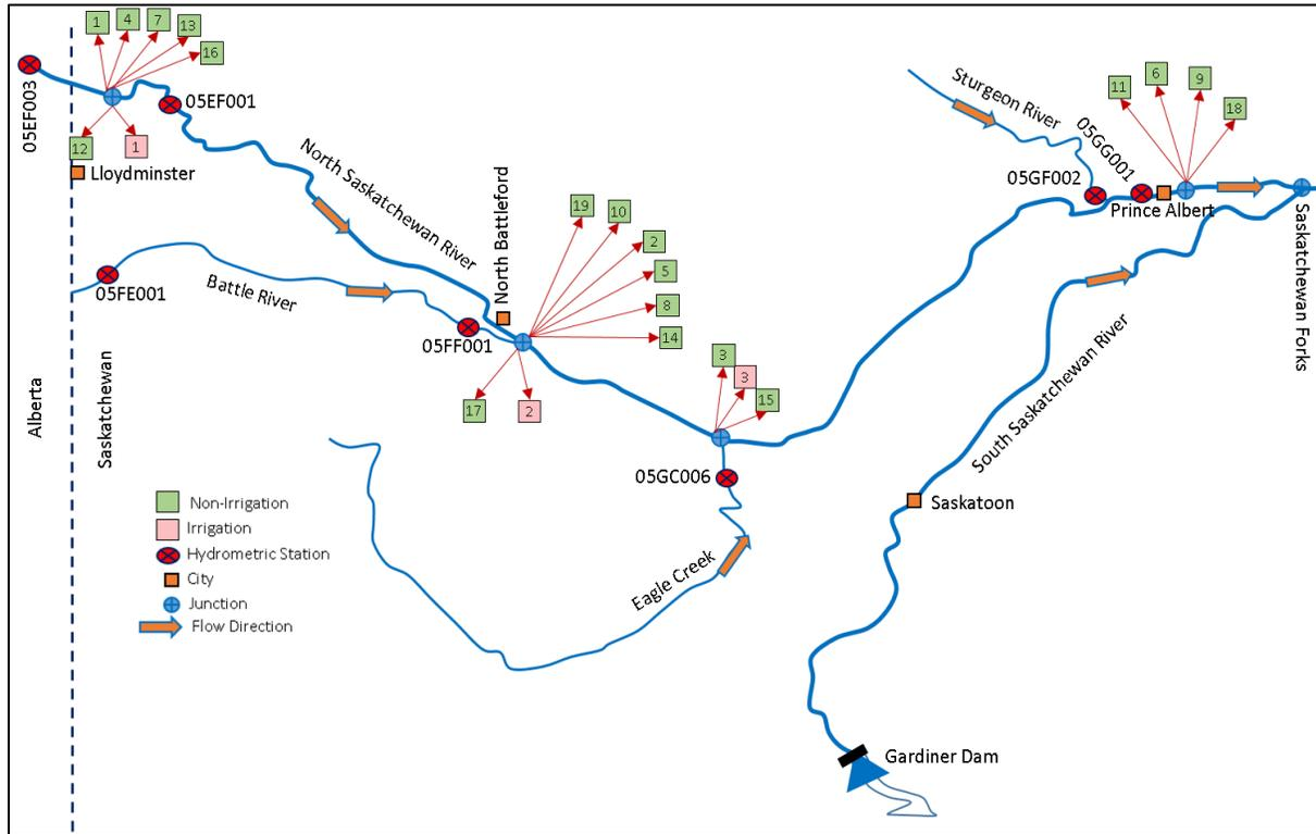
Figure G.1 Schematic of the North Saskatchewan River (NSR) basin water resources system in Saskatchewan, from the Alberta-Saskatchewan border to Prince Albert, Saskatchewan
