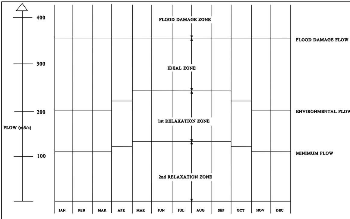
Figure A.2 Flow zones of natural channel in WRMM (Alberta Environment, 2002)
