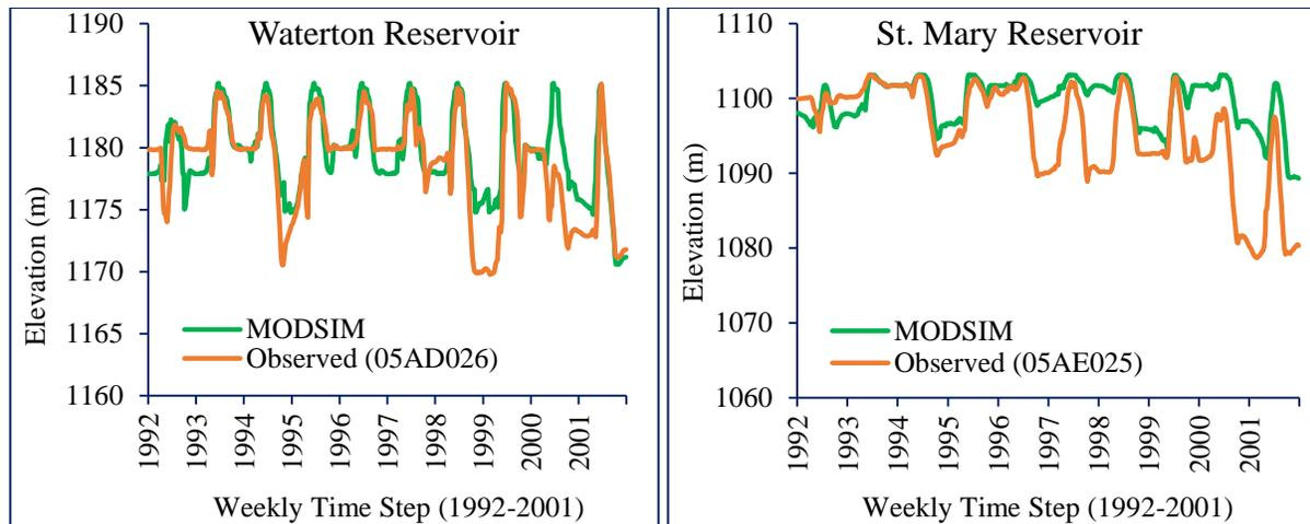
Figure E.10 Modsim simulation results for the Waterton and St. Mary reservoirs
