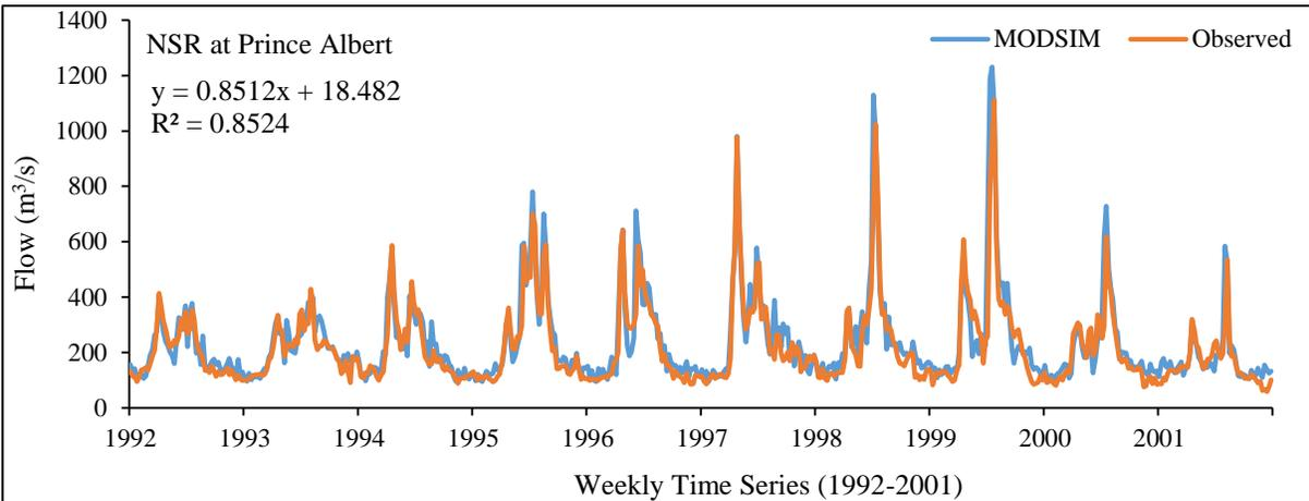
Figure G.4 MODSIM simulated streamflow for the NSR at Prince Albert, Saskatchewan
