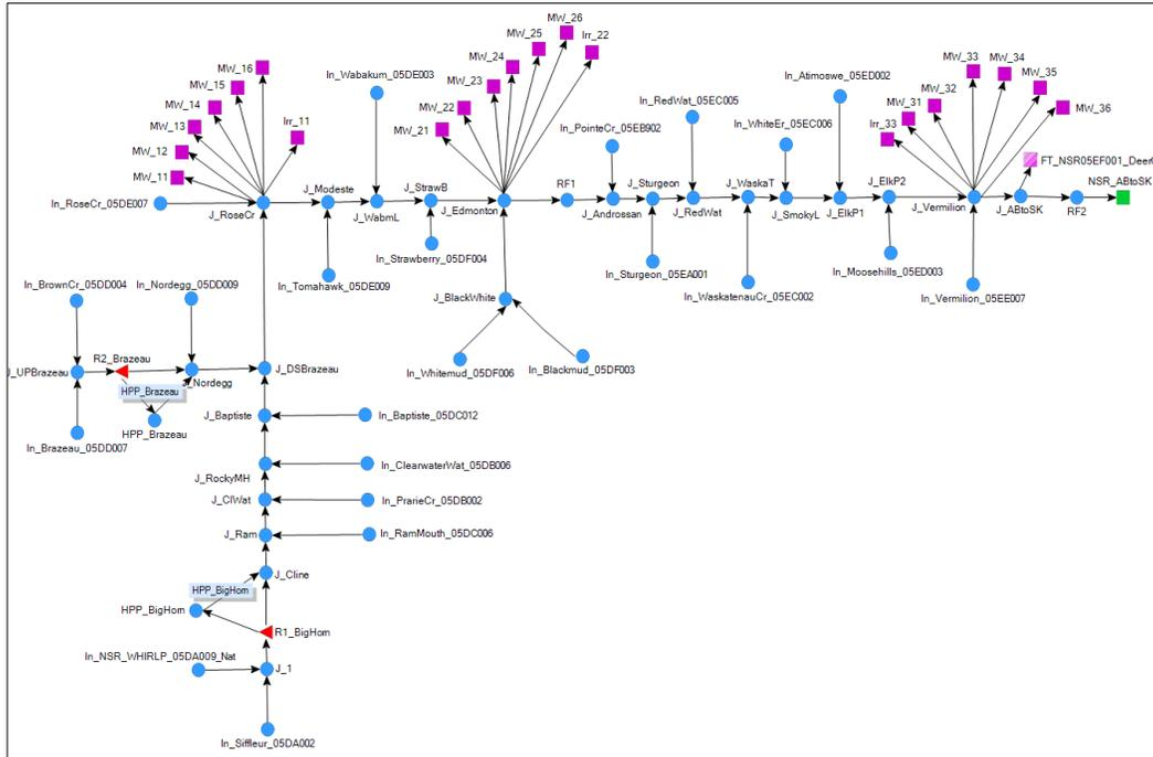
Figure F.5 Developed NSR-AB model schematic in MODSIM GUI
