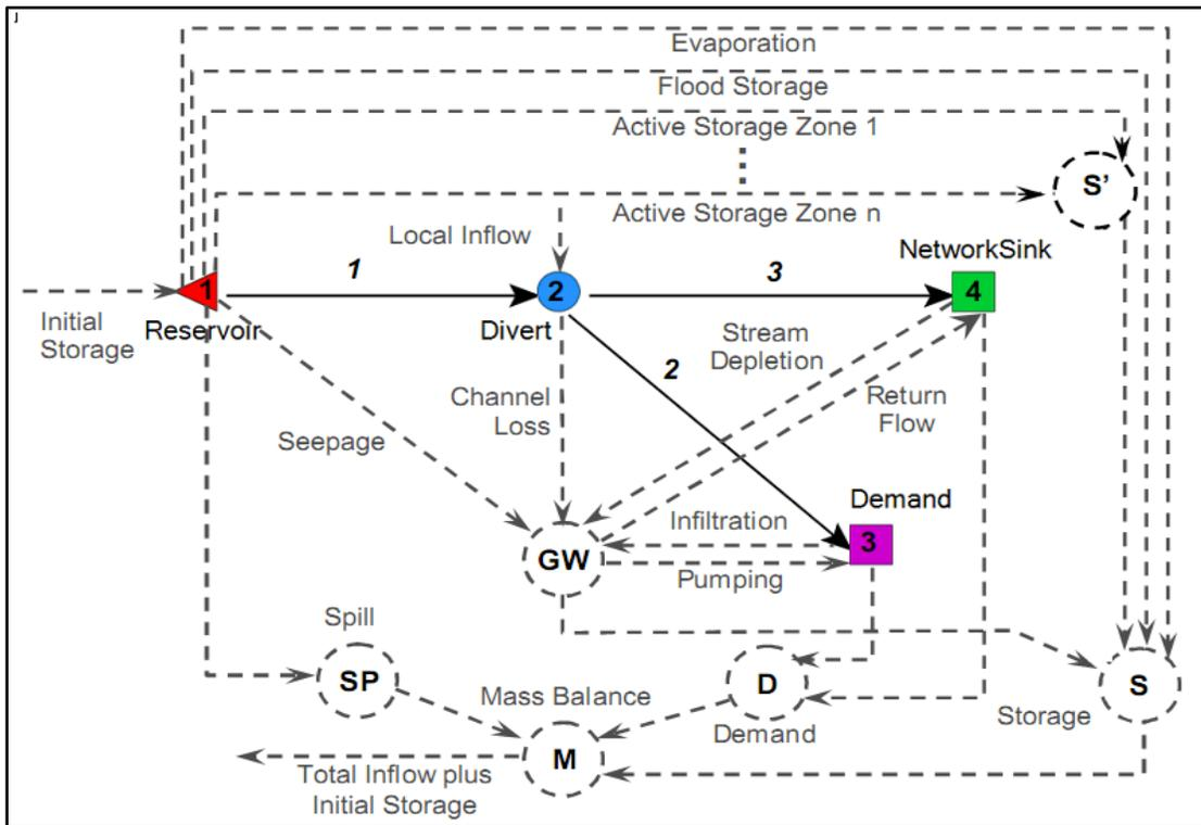
Figure A.5 MODSIM network structure with artificial nodes and links (Labadie and Larson, 2007)
