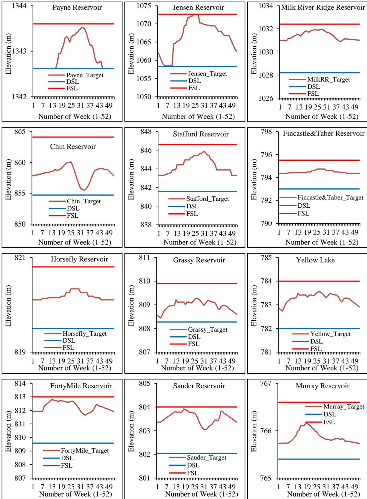
Figure E.3 Operating policy of different reservoirs considered in STRIBS model development
