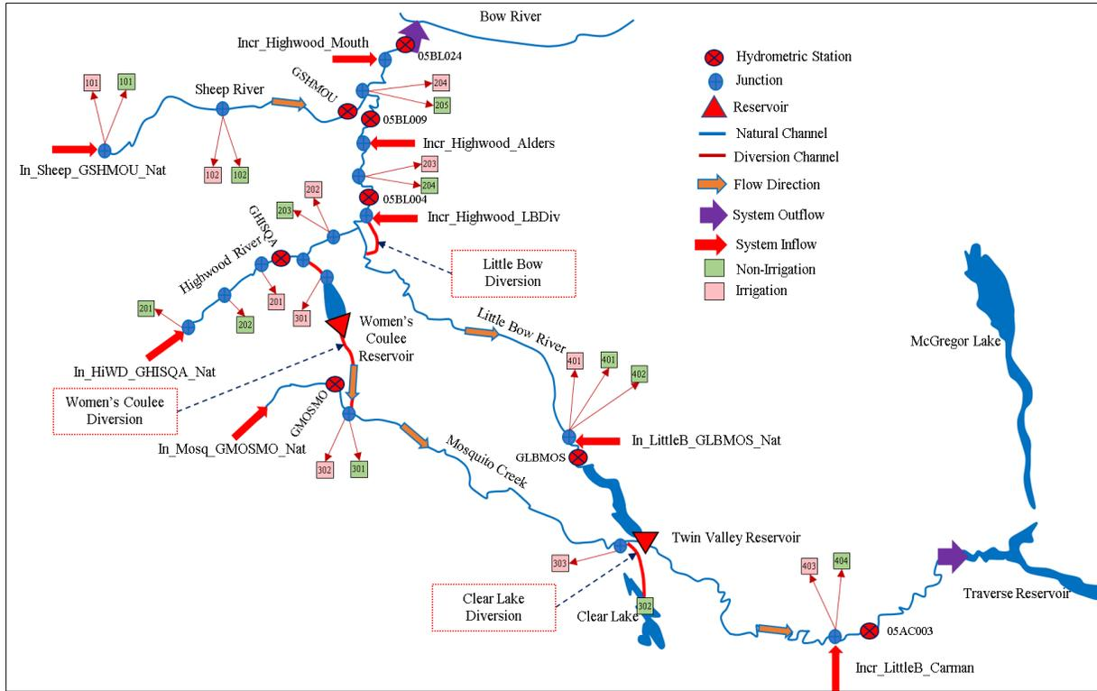
Figure D.1 The Highwood River Diversion Plan (HRDP) area located in the Upper Highwood and Upper Little Bow rivers
