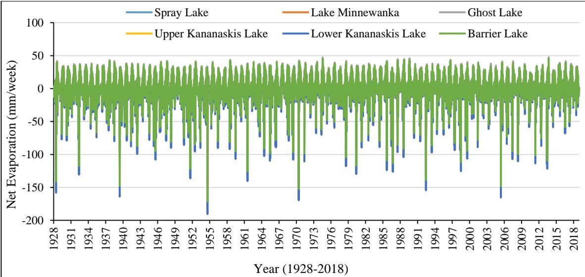
Figure C.3 Net reservoir evaporation considered in the TAU model development
