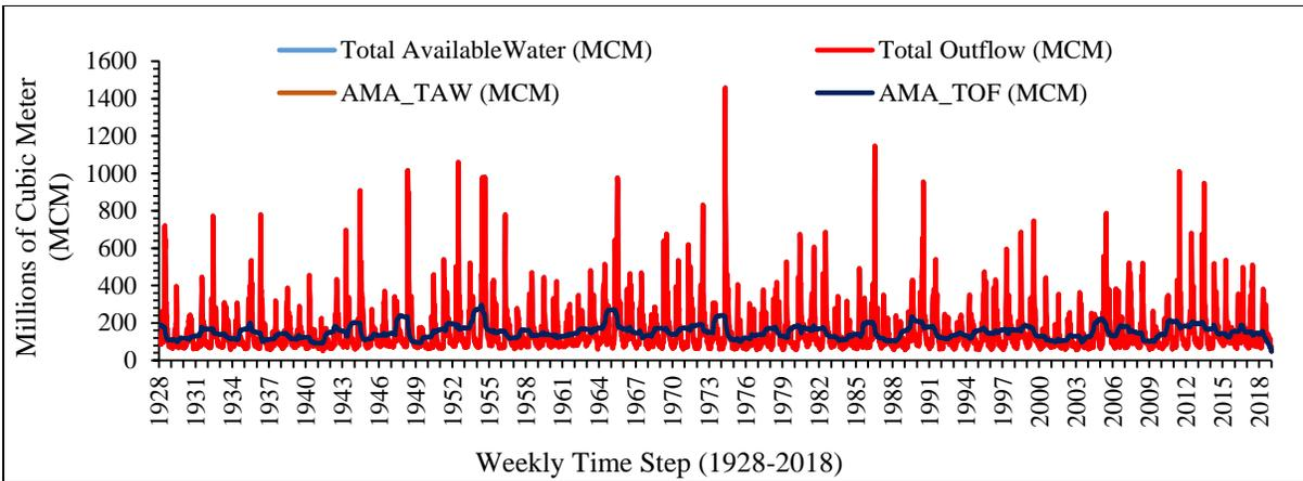
Figure G.3 Water balance of the developed NSR-SK model at each time step (weekly), and annual moving average (AMA) of total available water (TAW) and total outflow (TOF)
