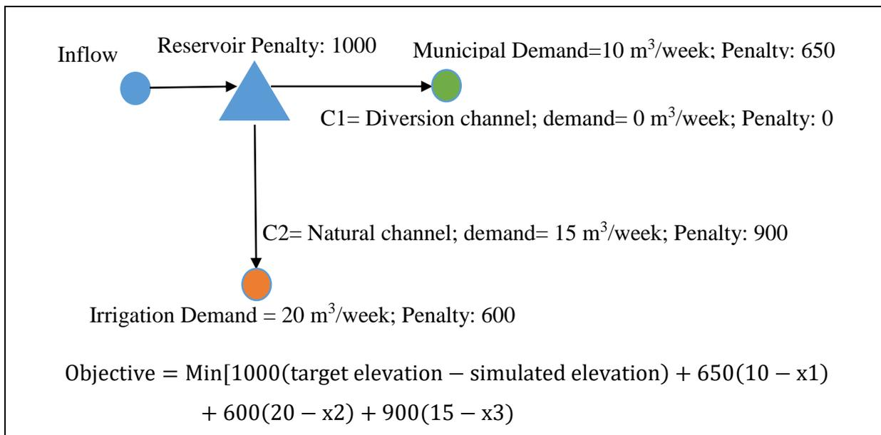
Figure A.4 A simple network that depicts WRMM problem formulation and objective function of water allocation
