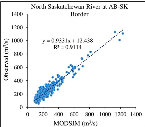
Figure F.6 Comparison between MODSIM simulated and observed streamflow for the North Saskatchewan River at Edmonton and Alberta (AB)-Saskatchewan (SK) border
