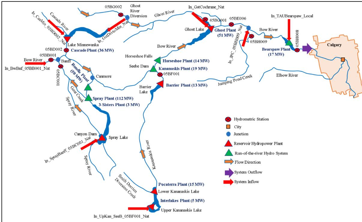
Figure C.1 Water resources system diagram of the TransAlta Utilities (TAU) located in the upstream of the Bow River, Alberta
