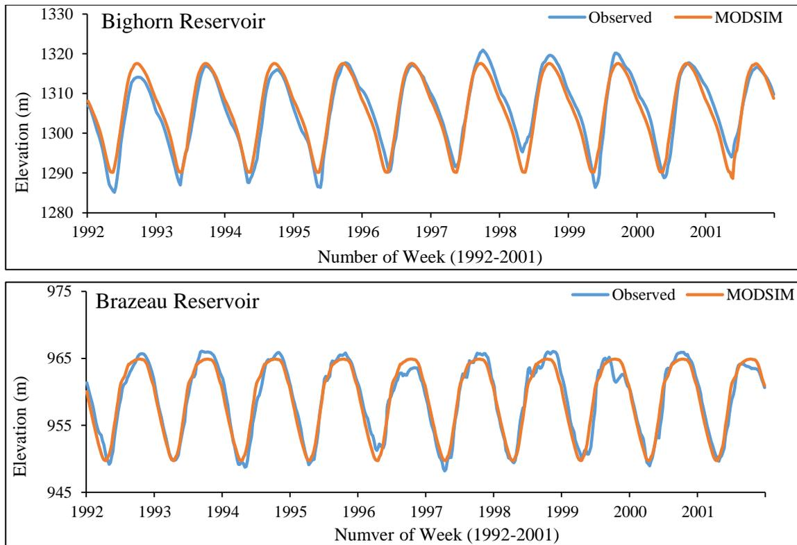
Figure F.7 MODSIM simulated elevation for the NSR-AB reservoirs
