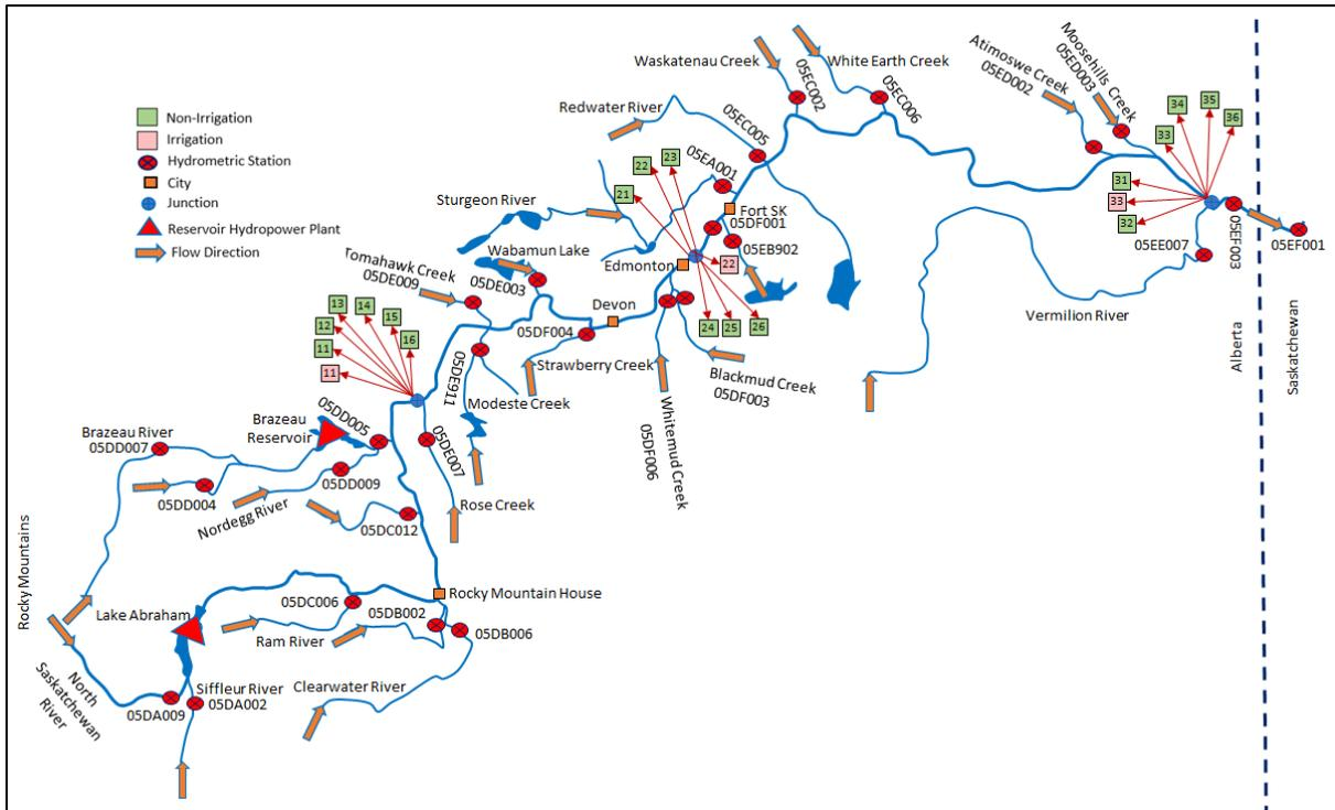
Figure F.1 Schematic of the water resources system of the North Saskatchewan River Basin in Alberta (NSR-AB) from the Rocky Mountains to the Alberta-Saskatchewan border
