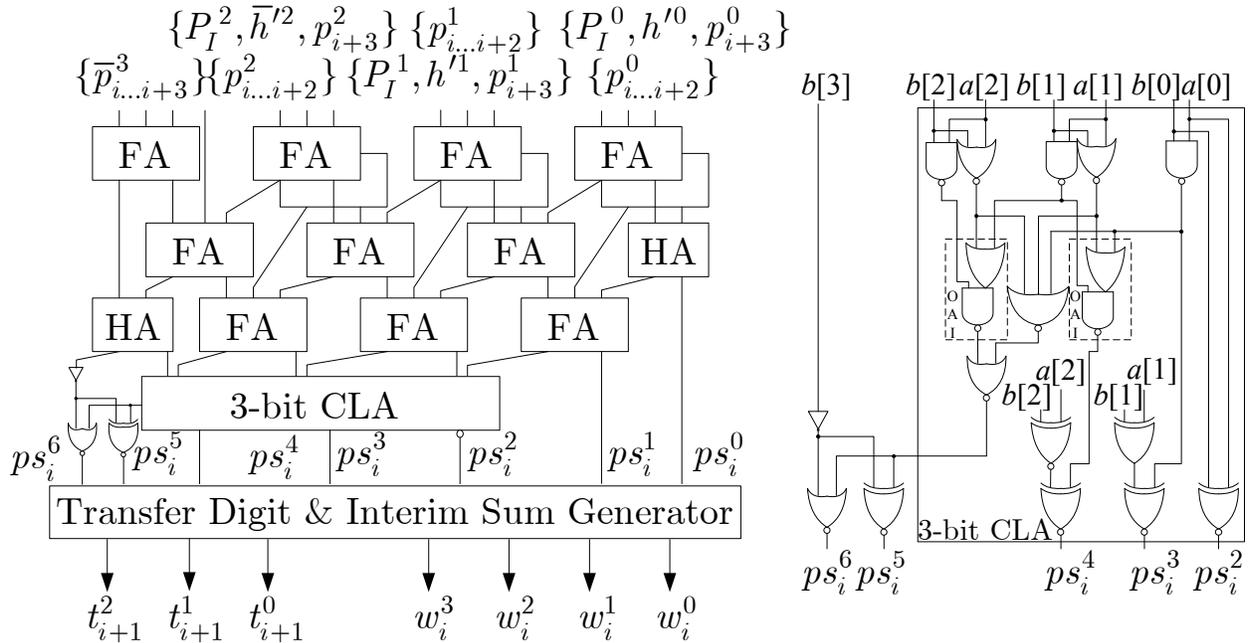
**Figure 6.9:** Hardware structure of the proposed 1<sup>st</sup> level multi-operand SD adder
