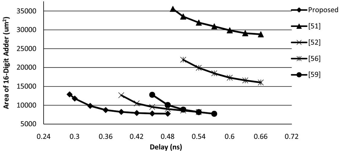
Figure 7.1: Area-Delay Comparison
