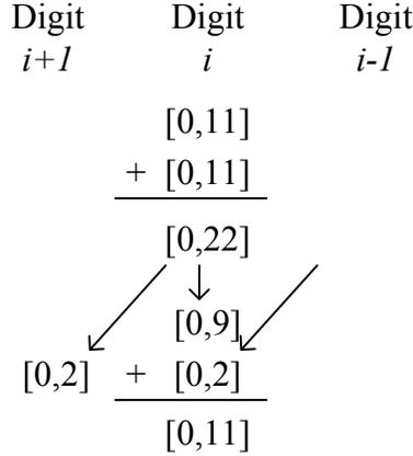
**Figure 4.1:** Example of calculation with redundant number system
