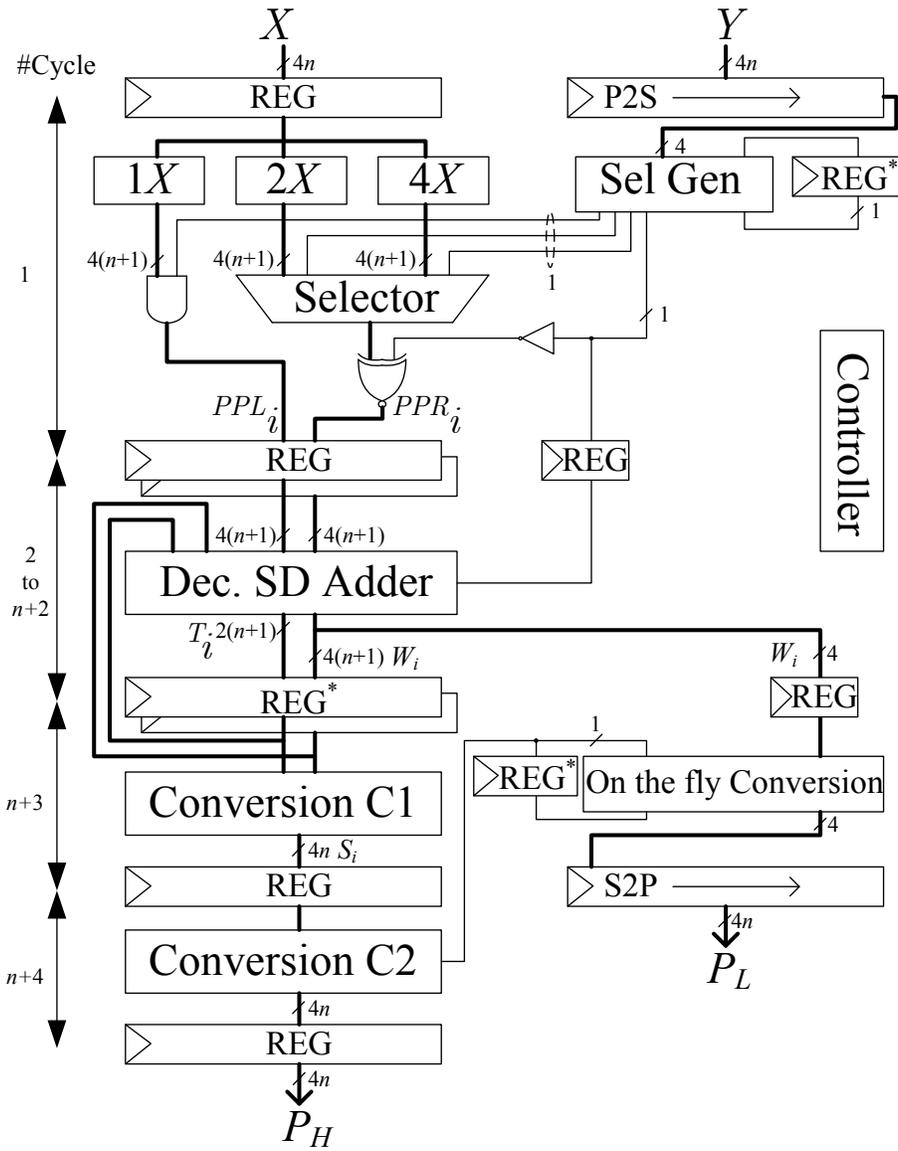
Figure 6.20: The proposed sequential decimal multiplier
