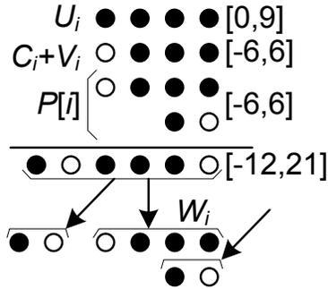
**Figure 6.17:** The dot-notation of partial product accumulation (digit-slice)
