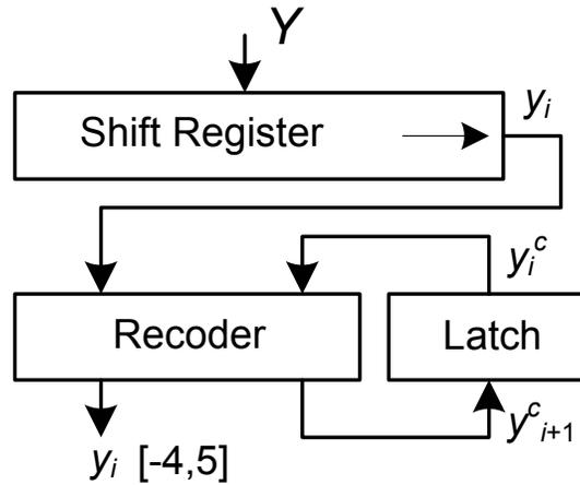
**Figure 6.15:** Recoding of the multiplier
