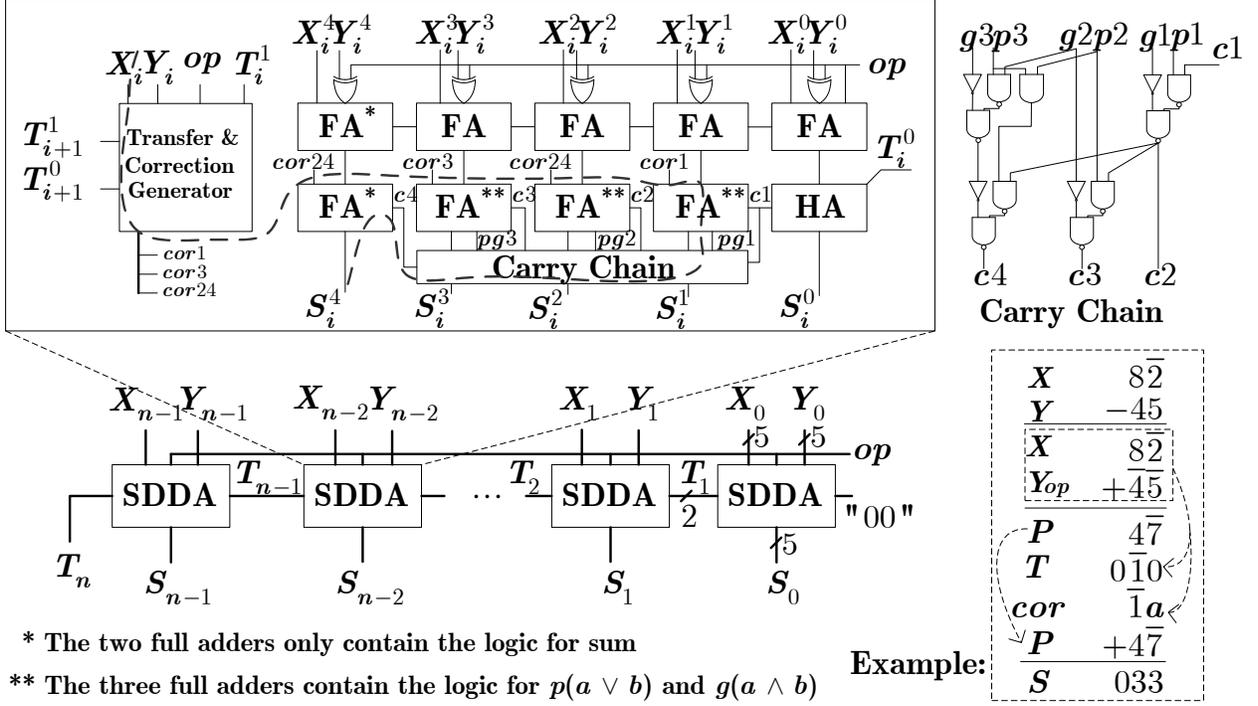
Figure 6.1: Proposed n-digit signed digit decimal adder
