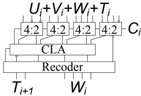
**Figure 6.18:** The circuitry of partial product accumulation (digit-slice)
