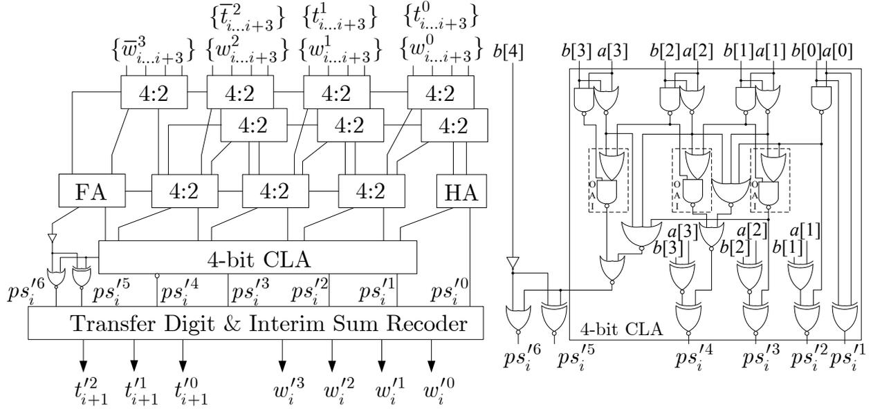
**Figure 6.10:** Hardware structure of the proposed 2<sup>nd</sup> level multi-operand SD adder
