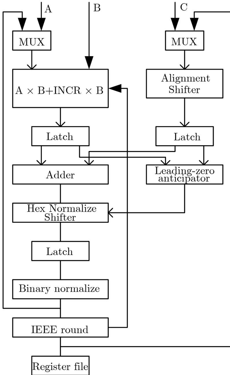
Figure 3.2: Binary FMA architecture of [26]
