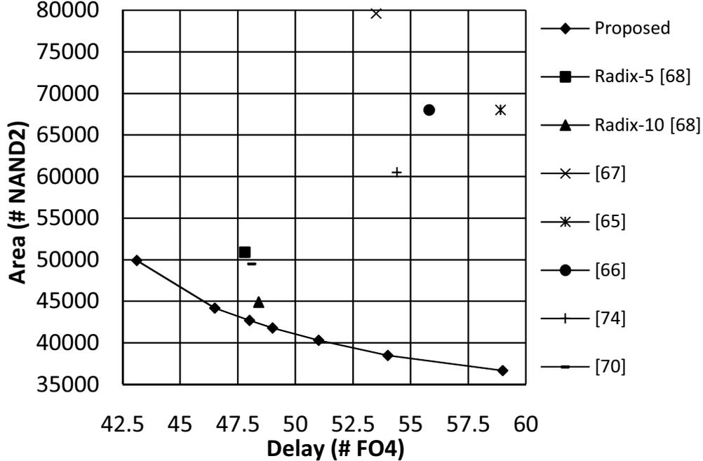
**Figure 7.3:** Delay-area space of the decimal multipliers
