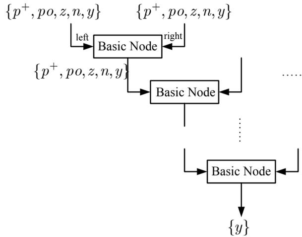
**Figure 6.30:** Hardware structure of the correction detection unit
