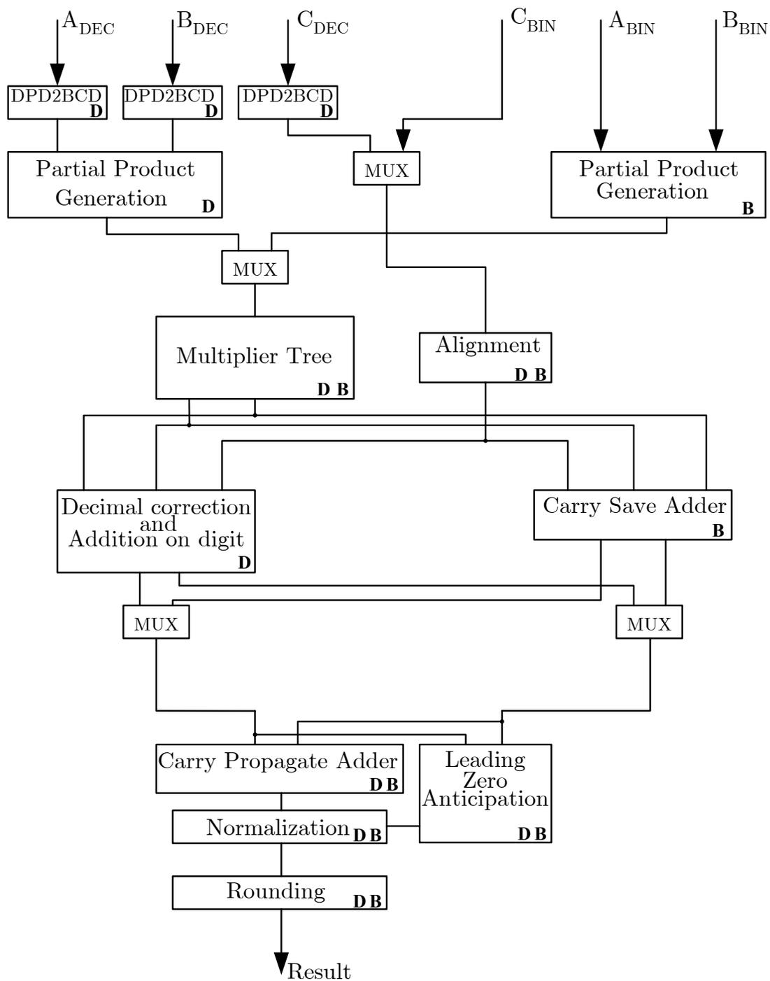
**Figure 3.5:** Combined Decimal and Binary FMA architecture
