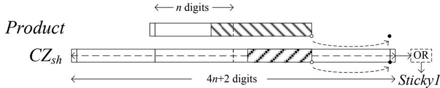
**Figure 6.27:** Layout of the aligned product and addend
