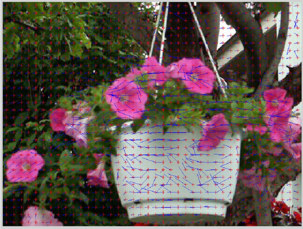
Figure 5.15 Motion Vectors between Frames 11 and 12 of a Rotating Flower Basket using Block Matching Method
