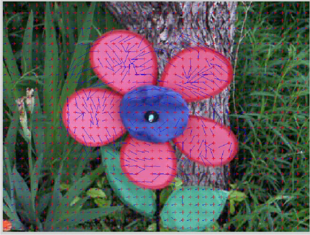
Figure 5.16 Motion Vectors between frames 23 and 24 of a Rotating Pinwheel using Block Matching Method
