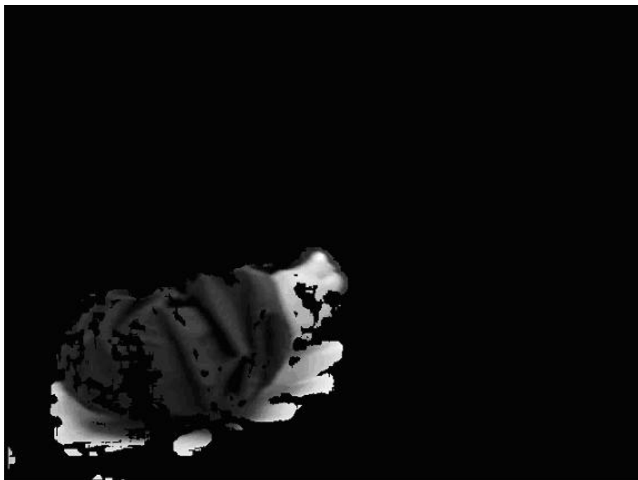
Figure 5.9 Segmentation of the moving arm using threshold value of 2.0
