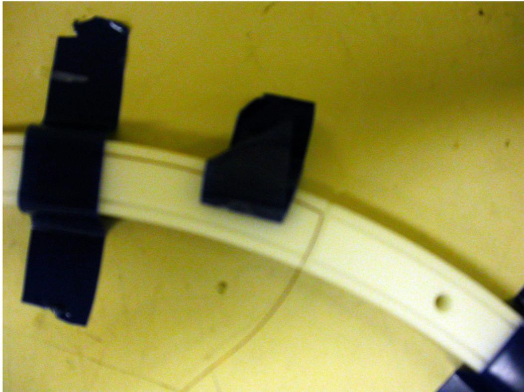
**Figure A.3:** Coil winding turning corners in the form grooves. A piece of tape is lifted to illustrate the winding method.
