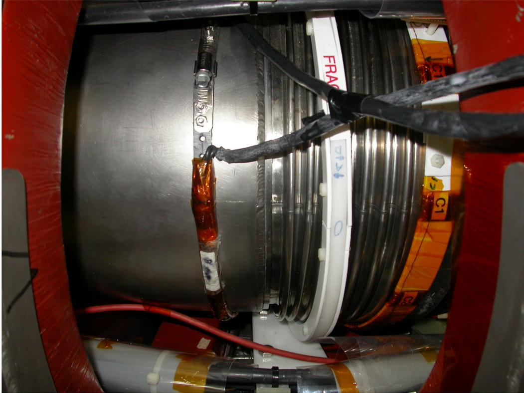
**Figure A.4:** Diamagnetic coil installed on STOR-M
