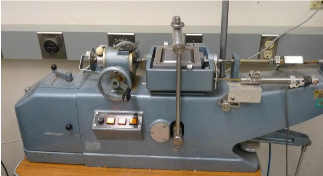
Figure 3.11 Shear box apparatus used for carrying out coefficient of internal friction test.
