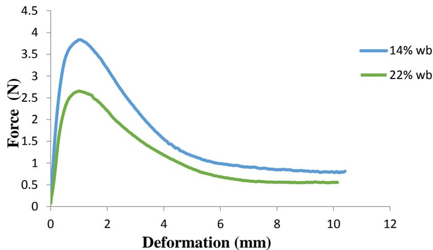
Fig. 4.7 Force-deformation curve of ‘Commander’ comparing forces needed to bend the stem at the first internode with 14 and 22% (wb) moisture content.
