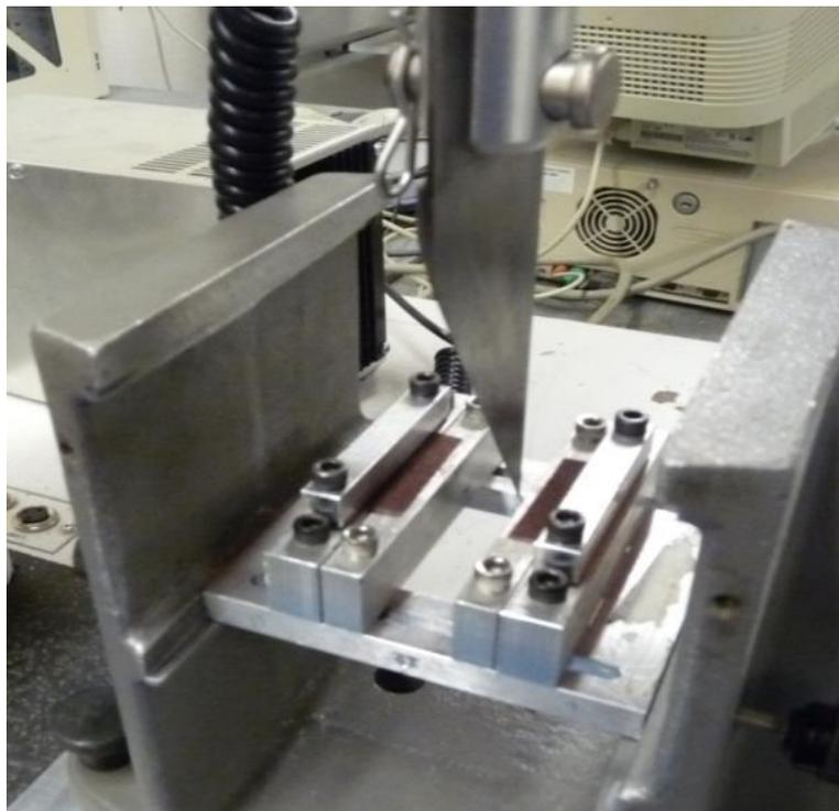
Figure 3.7 Cutting tool mounted on the Instron universal tester used for carrying out cutting test.
