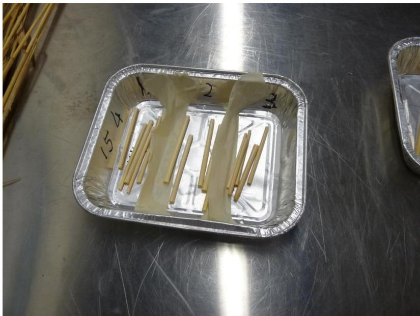
Figure 3.2 Sample preparation showing cut samples for further moisture adjustment and subsequent testing.
