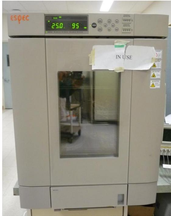
Figure 3.4 Espec environmental chamber used for moisture adjustment of sample before testing.
