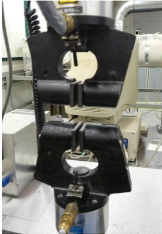
Figure 3.8 Hydraulic steel clamp with rubber fittings and emery paper glued for conducting tensile test.
