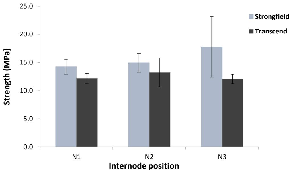
Fig. 4.5 Graph comparing stem shearing strength of ‘Strongfield’ and ‘Transcend’ at different internode with 18% (wb) moisture content.
