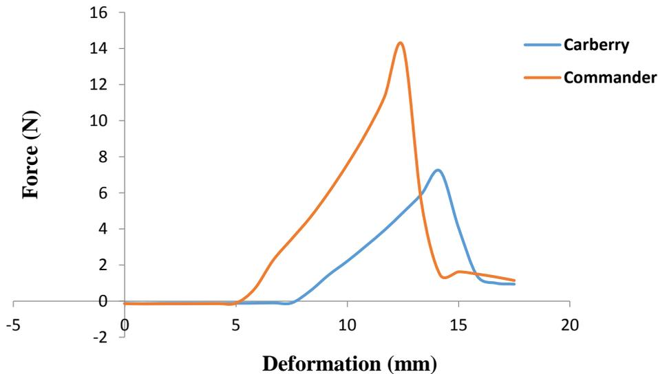
Fig. 4.6 Force-deformation curve comparing forces needed to cut the first internode of ‘Commander’ and ‘Carberry’ stem at 14%.
