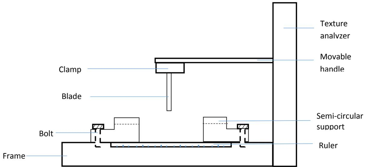
(a) Schematic diagram of the 3-point bending test tool. (Not to scale).
