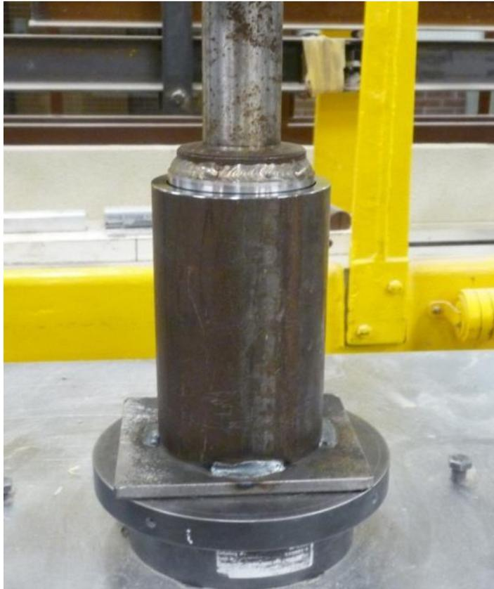
Fig. 3.12 Cylinder and plunger mounted on the INSTRON 600 DX for compression testing.
