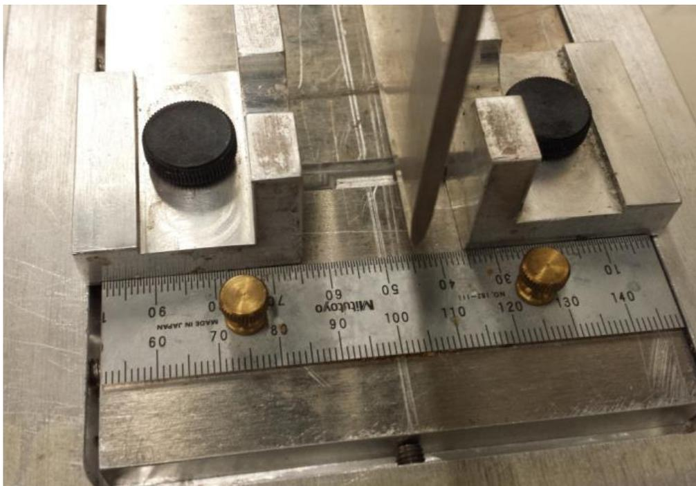
(b) Photograph of the three point bending test tool setup.
