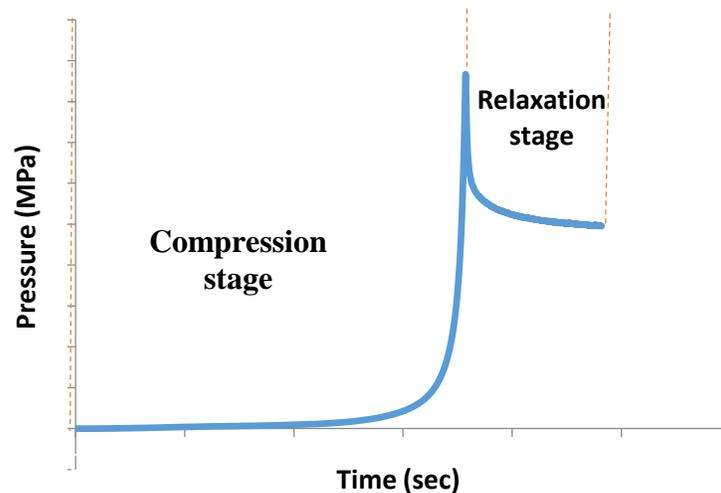
Fig. 3.13 Typical graph of pressure against time showing the compression and relaxation stages during compression test (redrawn from Talebi et al. 2011).
