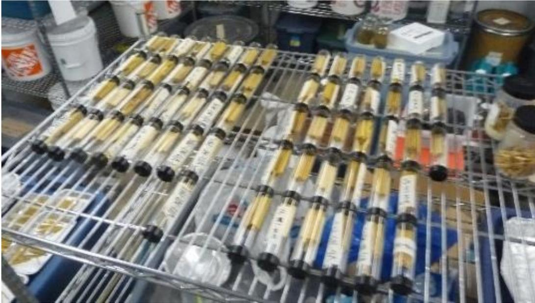
Figure 3.3 Samples were placed inside glass vials with cap and stored in a controlled climatic storage (4°C temperature and 30% relative humidity).
