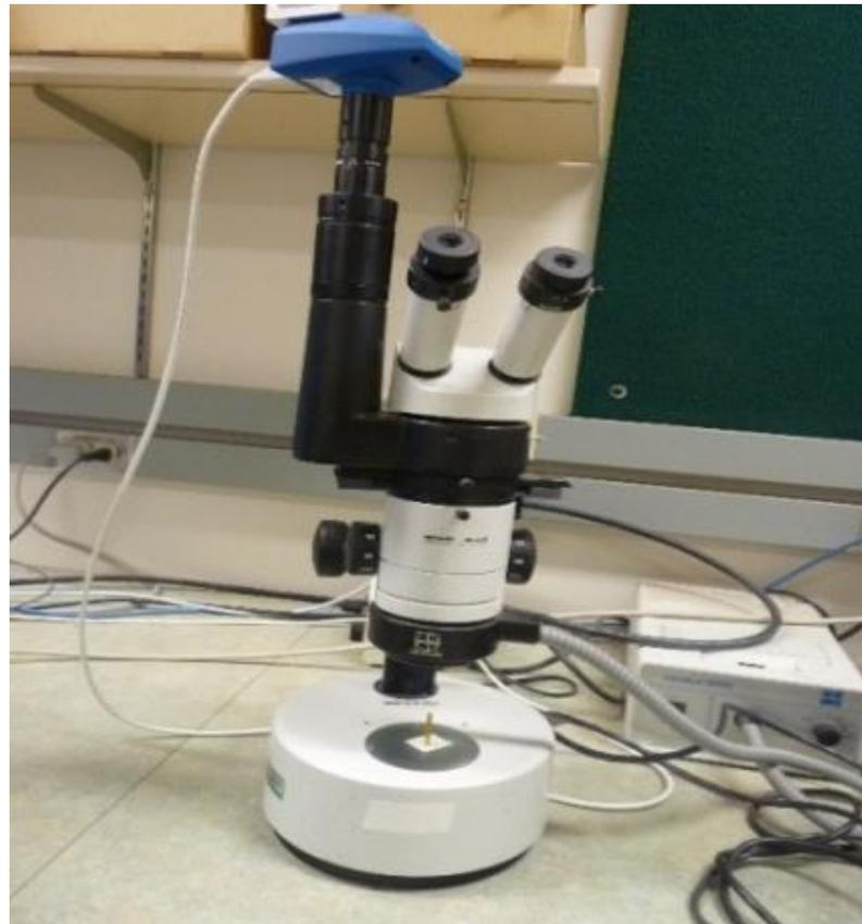
Figure 3.9 Wheat stem sample mounted on the Wild Herbrugg stereoscope during determination of stem diameter.
