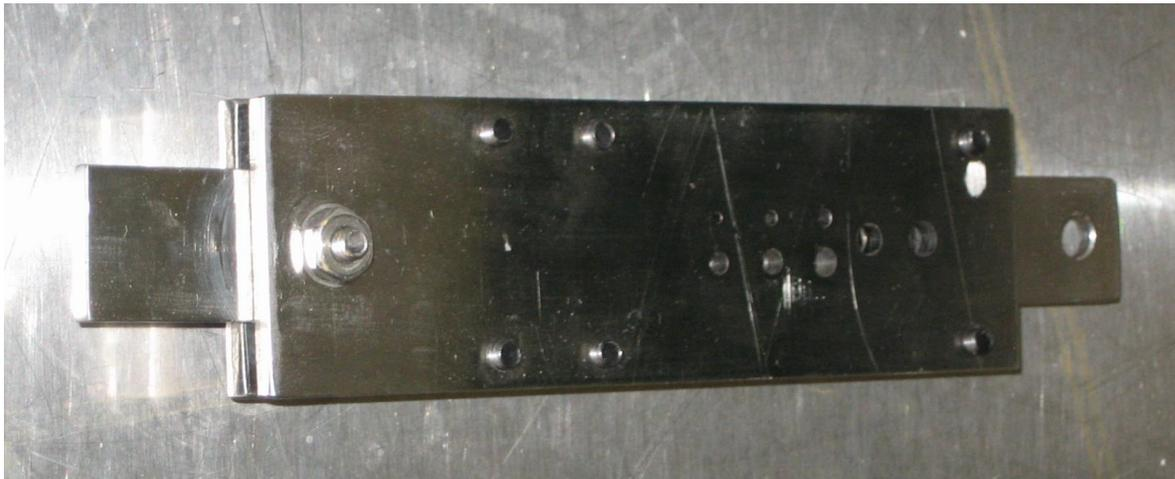
Figure 3.5 Shear tool used for shearing tests with sliding plate in the middle.
