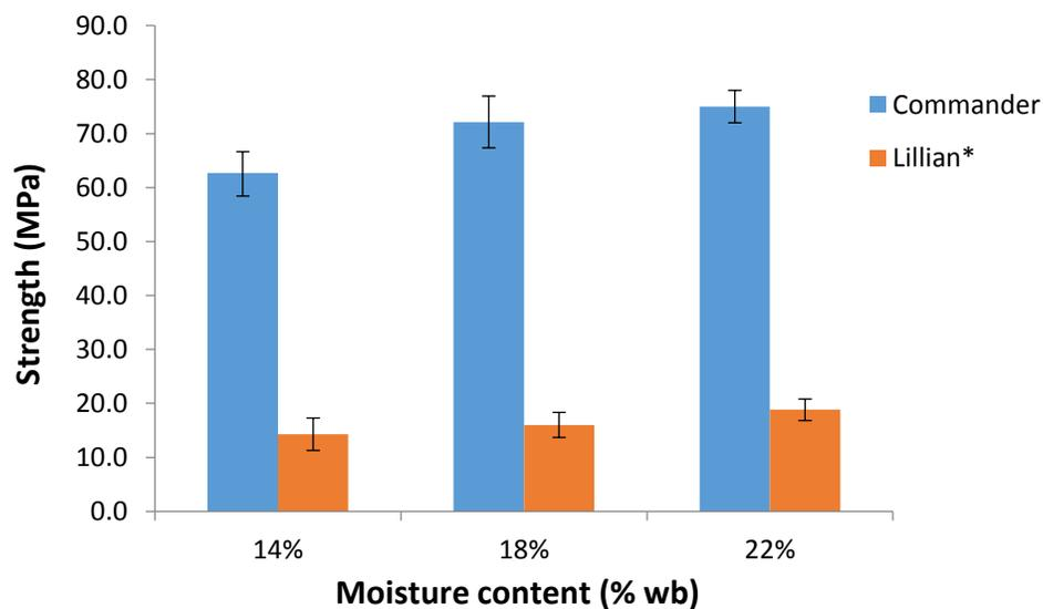
Fig. 4.8 Graph comparing stem tensile strength of ‘Commander’ and ‘Lillian’ first internode position at different moisture content (% wb).
