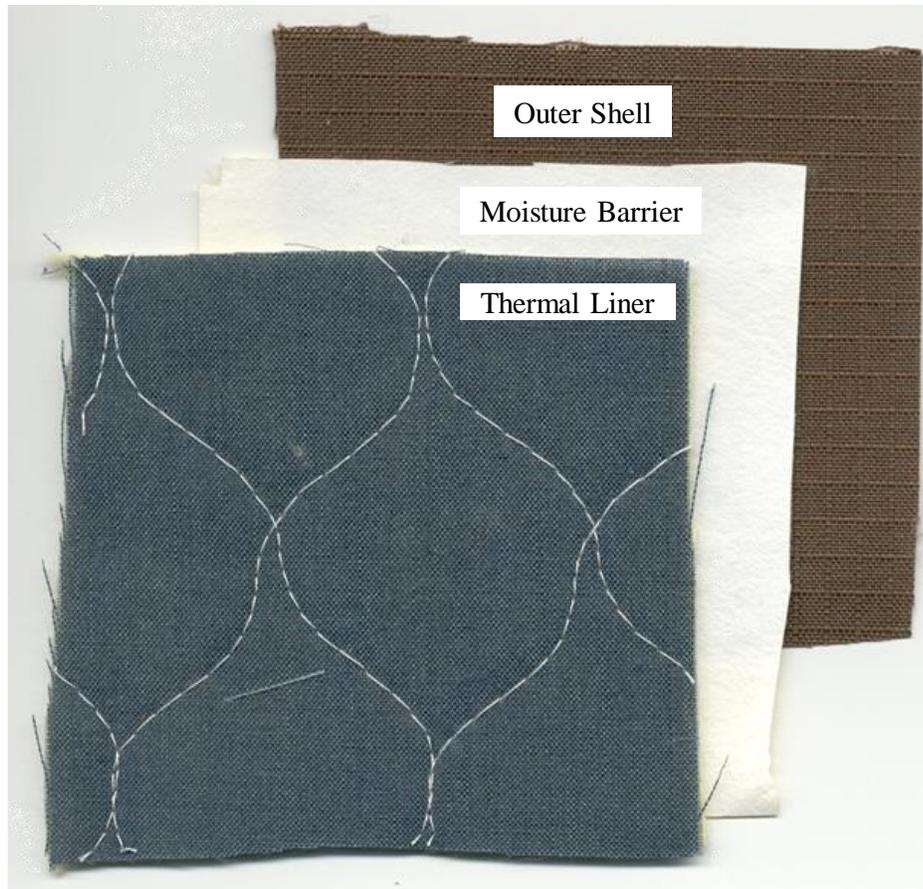
*Figure 1.1 Example of A Multilayer Ensemble For Fire Protective Garments (Rezazadeh 2014)*
