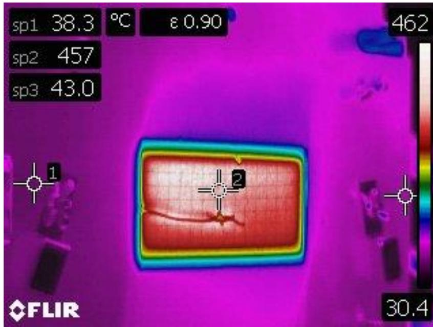
*Figure 2.12 FLIR Photo Of Ripstop Natural With Thermocouple And Off Gassing*
