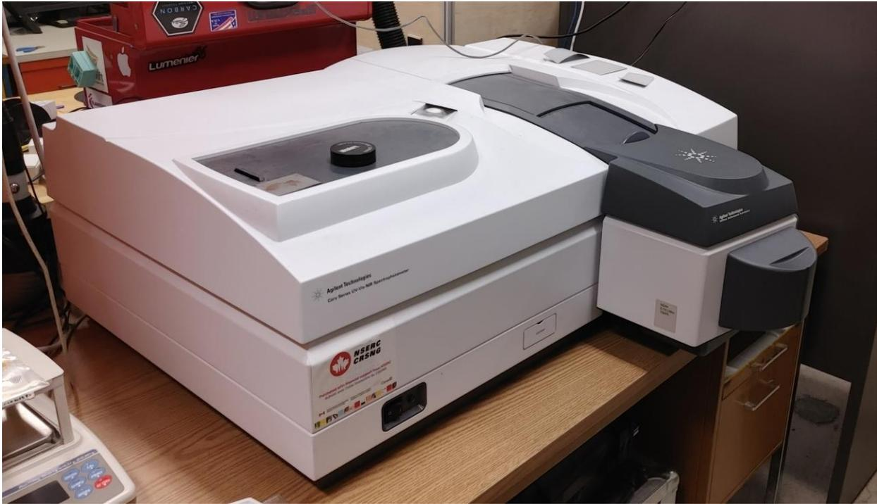
*Figure 2.13 The Agilent Technologies Cary Series UV-VIS-NIR Spectrophotometer*
