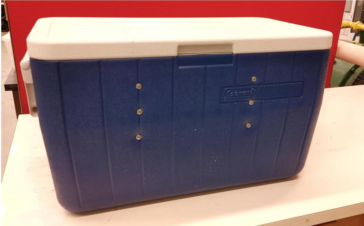
*Figure 2.5 The Conditioning Chamber Used For Preparing The Specimens For Thermal Exposure*
