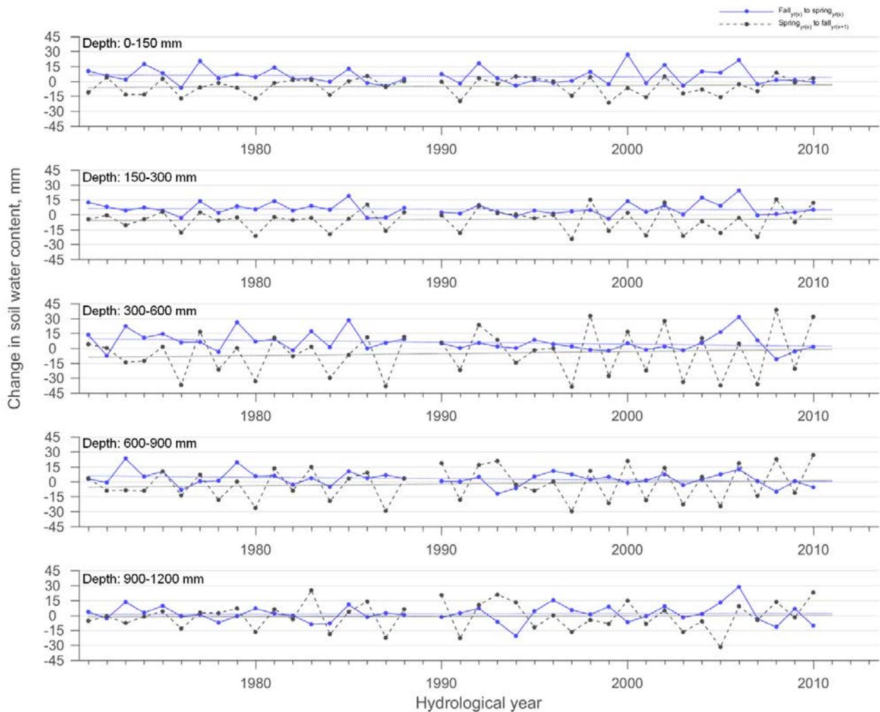
**Figure 2.8** Change in hillslope-averaged seasonal soil water content (mm) for Hillslope 3 for five depth layers (0-150 mm, 150-300 mm, 300-600 mm, 600-900 mm, 900-1200 mm below the soil surface) for fall to spring (over winter and snowmelt; blue) and spring to the following fall (over summer; grey). Trendlines are indicated.
