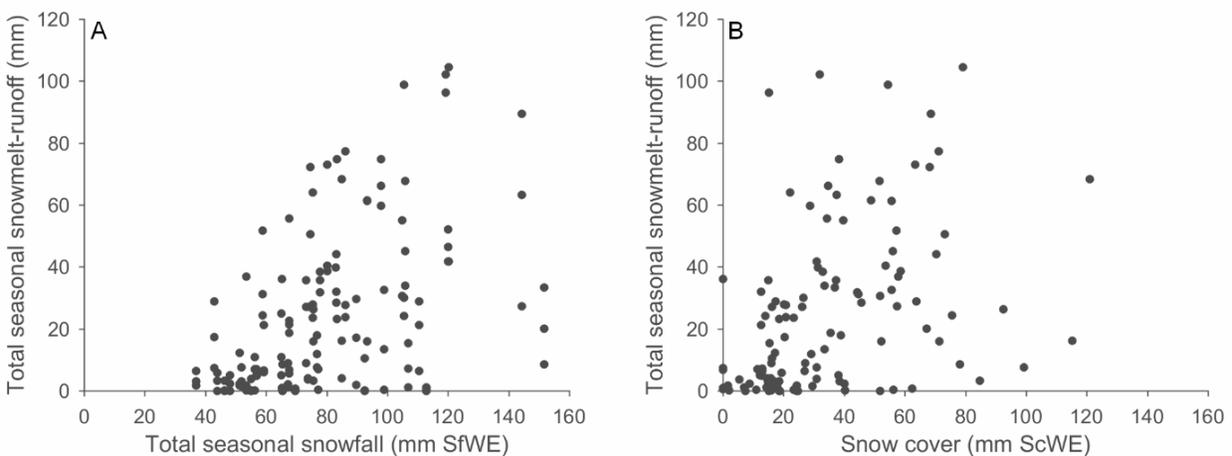
**Figure 3.2** Spring snowmelt-runoff events on the Swift Current hillslopes, showing A) the relationship between total seasonal snowfall (mm SfWE) and total seasonal snowmelt-runoff (mm); and B) the relationship between snow cover (mm ScWE) and total seasonal snowmelt-runoff (mm).
