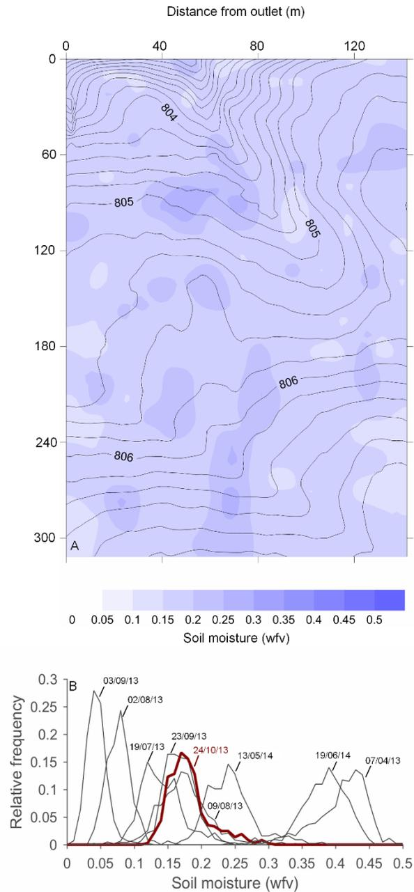
**Figure 4.6** (A) Spatial map of pre-freeze up soil surface water content (0-6 cm), measured on 24<sup>th</sup> October 2013; and (B) frequency distributions of all soil water content surveys conducted, with 24<sup>th</sup> October 2013 survey highlighted in red. Note that the colour scale of the spatial map (A) is the same extent as the x-axis of the frequency distributions in (B).
