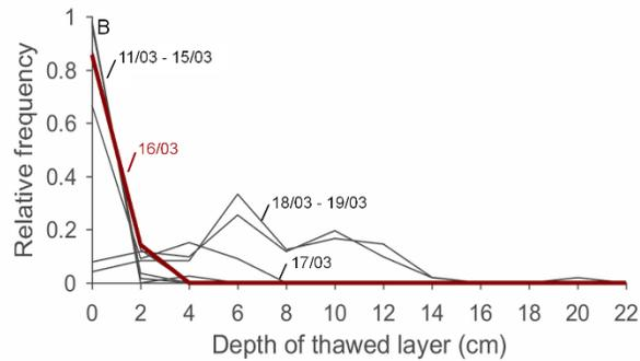
**Figure 4.5** (A) Spatial map of thawed layer depth on the day of peak snowmelt and peak runoff (16<sup>th</sup> March 2014); and (B) frequency distributions of all thawed layer depth surveys conducted, with 16<sup>th</sup> March 2014 survey highlighted in red. Note that the colour scale of the spatial map (A) is the same extent as the x-axis of the frequency distributions in (B).
