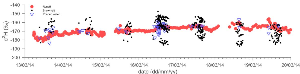
**Figure 4.7** Time series of stable isotopes (for  $\delta^2\text{H}$ ) of runoff, snowmelt, and ponded water through the snowmelt season. Pre-event  $\delta^2\text{H}$  soil water values measured on 20/02/14 (not shown) range between -112‰ and -140‰.
