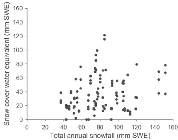
**Figure 2.6** Total annual snowfall (mm) and snow cover water equivalent (mm) measured before the onset of spring snowmelt for each year and each hillslope over the period 1965-2013.
