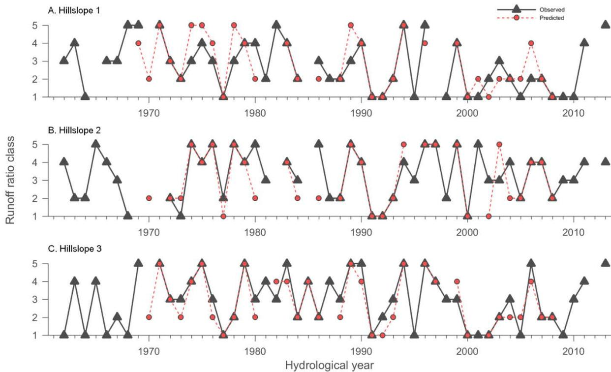
**Figure 3.4** Time series of observed runoff ratio classes (response variable) and predicted runoff ratio classes (predicted by the primary decision tree) for A) Hillslope 1, B) Hillslope 2, and C) Hillslope 3.
