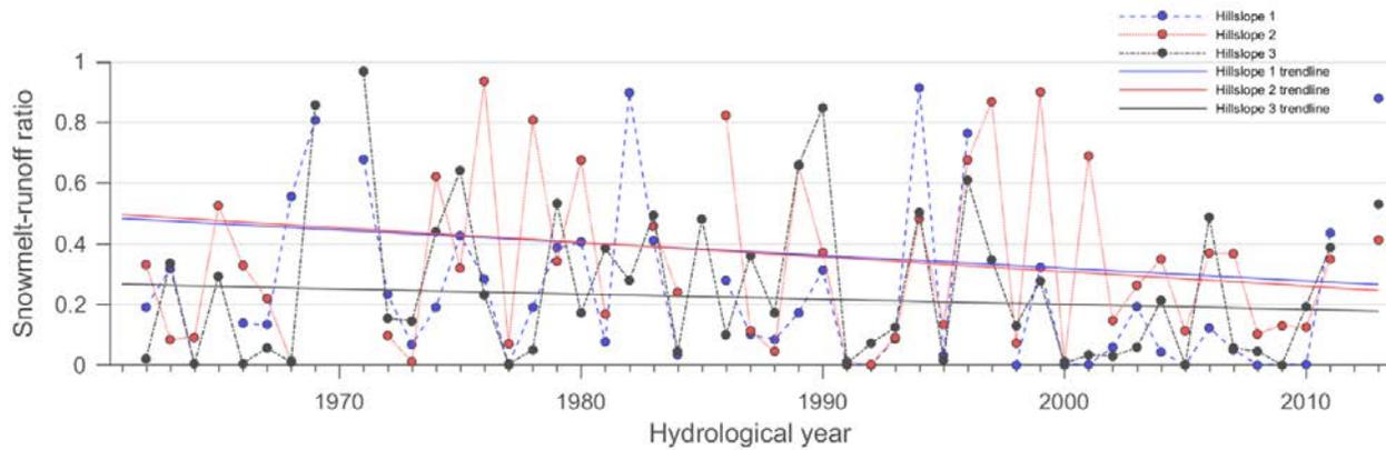
**Figure 2.9** Snowmelt-runoff ratio for each hillslope, where runoff ratio is calculated as snowmelt-runoff divided by total snowfall. Trendlines are indicated.
