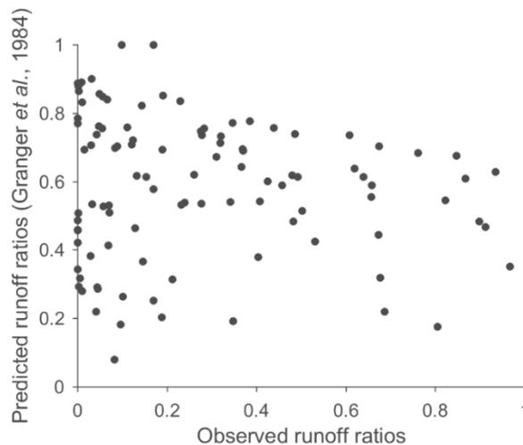
**Figure 3.7** Observed and predicted runoff ratios over the 1971-2013 period. The predicted runoff ratios were calculated using Equation 3.2, based on Granger's *et al.* (1984) empirical equation for infiltration into frozen ground.
