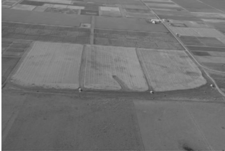
**Figure 3.1** Aerial photograph (facing south) of the Swift Current hillslopes (from right to left: Hillslope 1, Hillslope 2, Hillslope 3), taken in a year when wheat was grown. The three small heated huts at the northwest corners of the hillslopes, which house the runoff-monitoring equipment, are visible. Photograph reproduced, with permission, from Cessna *et al.* (2013).
