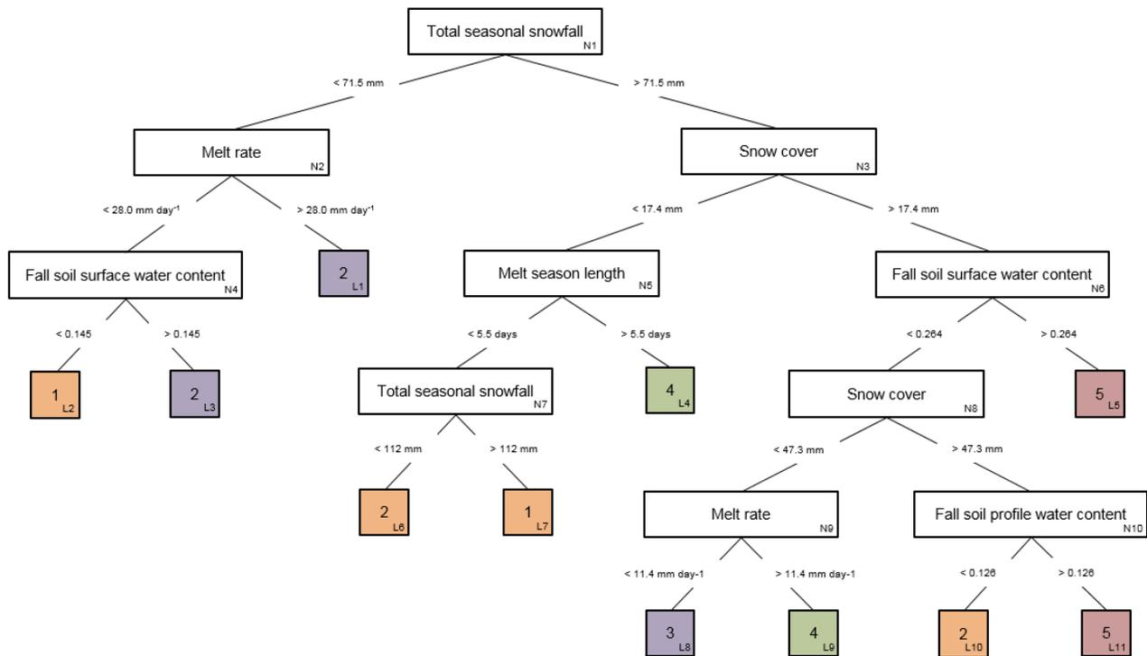
**Figure 3.3** Primary decision tree for predicting runoff ratios. The tree shows the variables used to explain runoff ratio, located at the nodes (N1, N2, etc.; white boxes) and the resultant predicted runoff ratio class at the leaves at the ends of each branch (L1, L2, etc.; coloured boxes). Table 3.3 gives the runoff ratio class data at each node and leaf, and the predictive accuracy at each leaf. The leaf colours are in reference to Figure 3.5.
