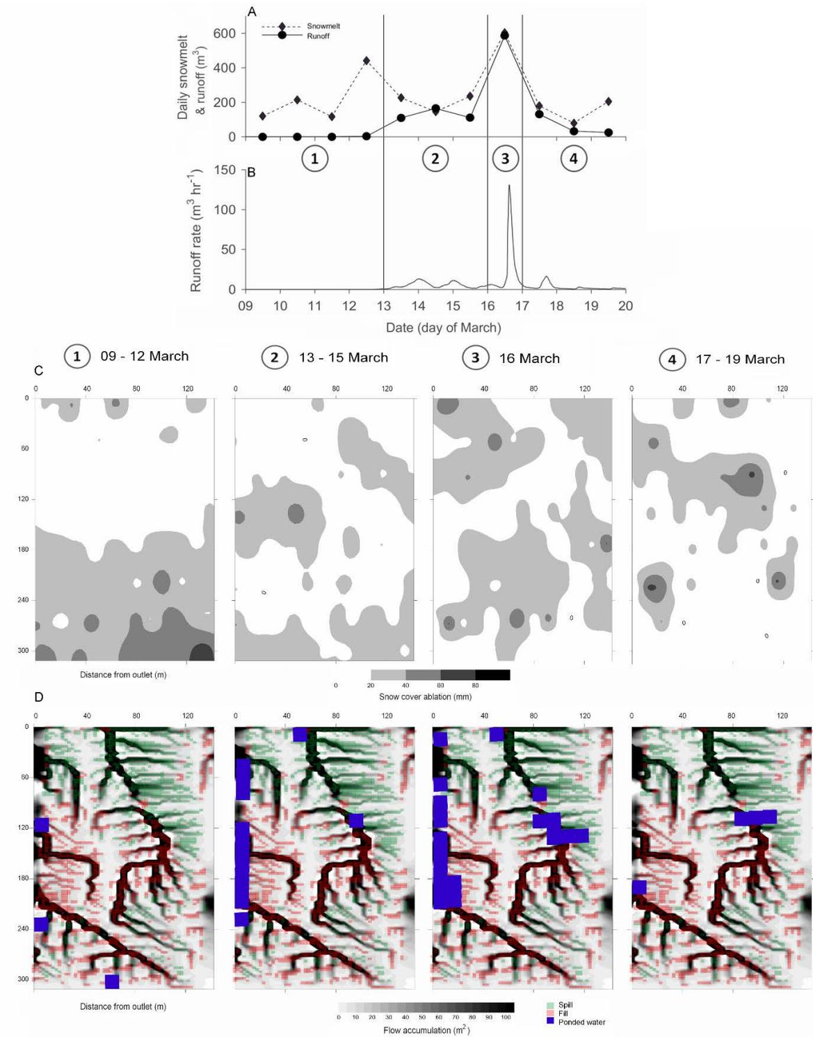
**Figure 4.3** For the 2014 spring snowmelt season on Hillslope 2: (A) daily snowmelt and runoff volumes and (B) runoff rates, recorded at 15-minute intervals. Four stages (1-4) are identified in the snowmelt-runoff, referred to in the text. Maps relate to each of these stages: (C) snowmelt over the hillslope for each stage; and (D) ponded water locations during each stage overlaid on fill and spill locations and the flow accumulation map.
