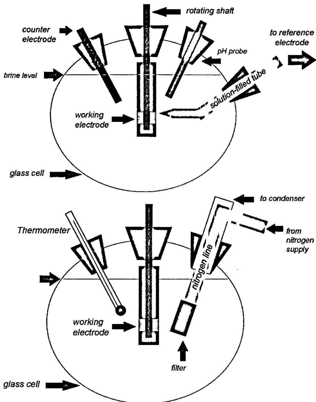
Figure 3.1b and 3.1c One Litre Bench Top Glass Cell, Side Views
