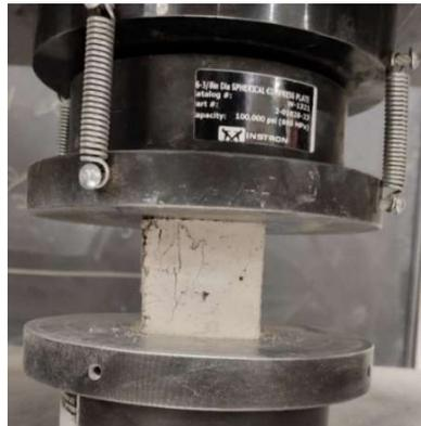
**Figure 3.13: Mortar Cube Test Setup**
