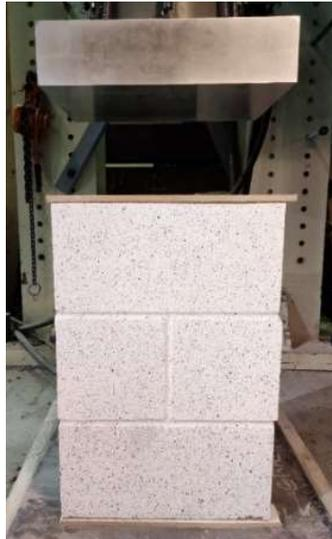
**Figure 3.11: Prism Positioned in the Test Setup**
