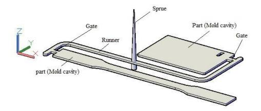
Fig. 4.2 Injection mold used in experiments including the delivery system and molded parts.
