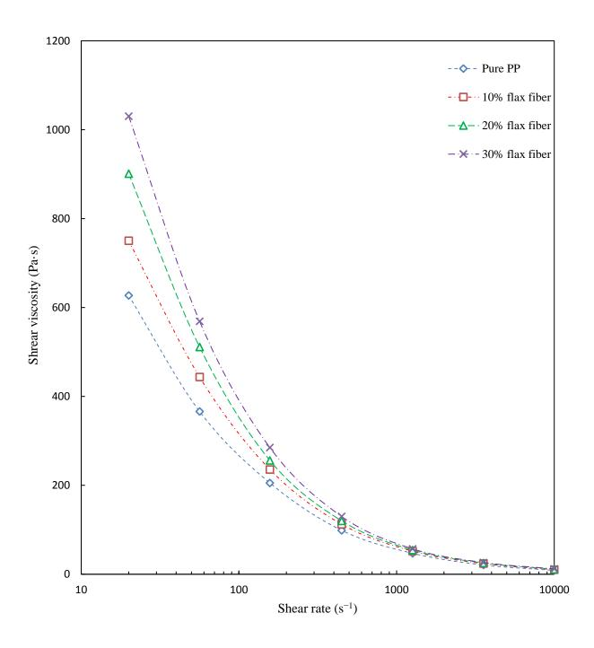
Fig. 4.4 Shear viscosity of pure PP and biocomposites at 220 °C as a function of the shear rate.
