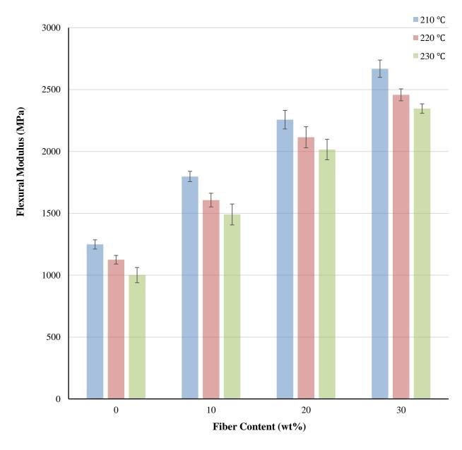
Fig. 3.22 The variation of flexural modulus of biocomposites with fiber contents and injection temperatures at injection pressure = 7.0 MPa.
