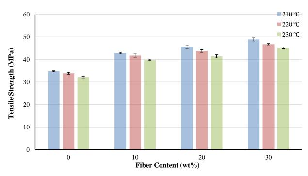
Fig. 3.10 The variation of tensile strength of biocomposites with fiber contents and injection temperatures at injection pressure 5.9 MPa.
