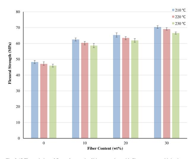
Fig. 3.17 The variation of flexural strength of biocomposites with fiber contents and injection temperatures at injection pressure = 4.8 MPa.
