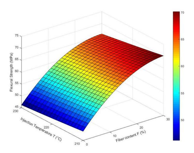
Fig. 3.23 The variation of flexural strength of biocomposites with flax fiber content and injection temperature by the predicted model of flexural strength.
