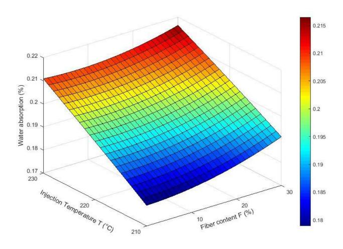
Fig. 3.28 The variation of water absorption of biocomposites with flax fiber content and injection temperature by the predicted model of water absorption.
