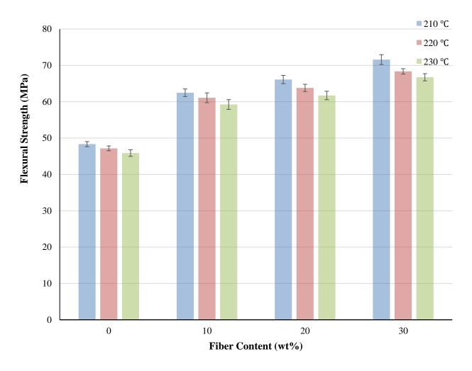
Fig. 3.21 The variation of flexural strength of biocomposites with fiber contents and injection temperatures at injection pressure = 7.0 MPa.
