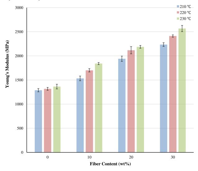
Fig. 3.12 The variation of Young's modulus of biocomposites with fiber contents and injection temperatures at injection pressure 4.8 MPa.
