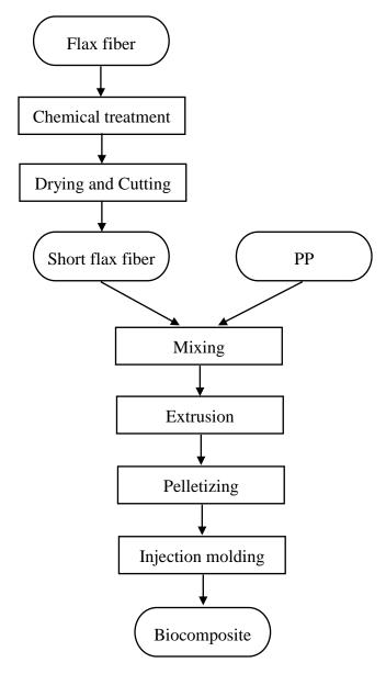
Fig. 3.1 Processing scheme of flax fiber reinforced PP Biocomposites.
