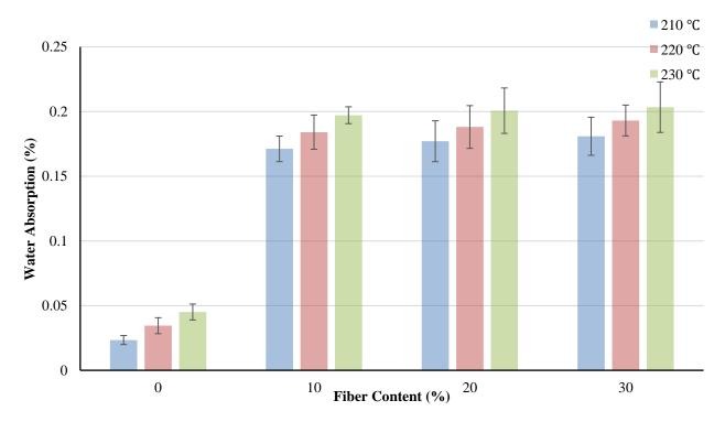
Fig. 3.25 The variation of water absorption of biocomposites with fiber contents and injection temperatures at injection pressure = 4.8 MPa.
