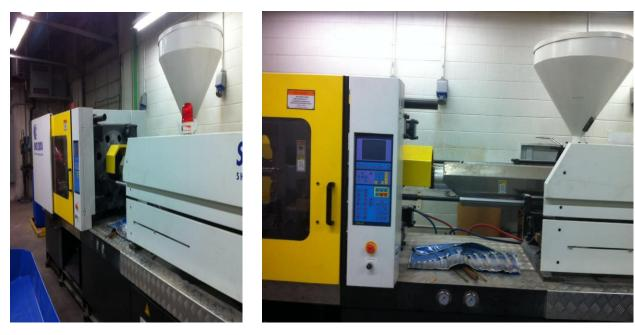
Fig. 3.5 Injection molding machine for producing biocomposites.
