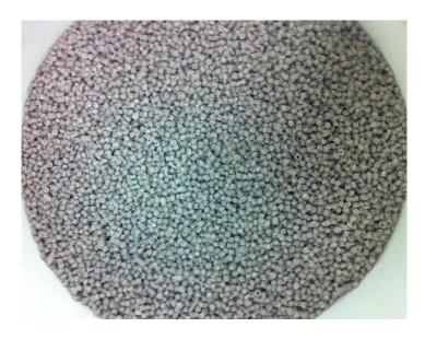
Fig. 3.3 The pellets of extruding the mixture of flax fibers and PP.
