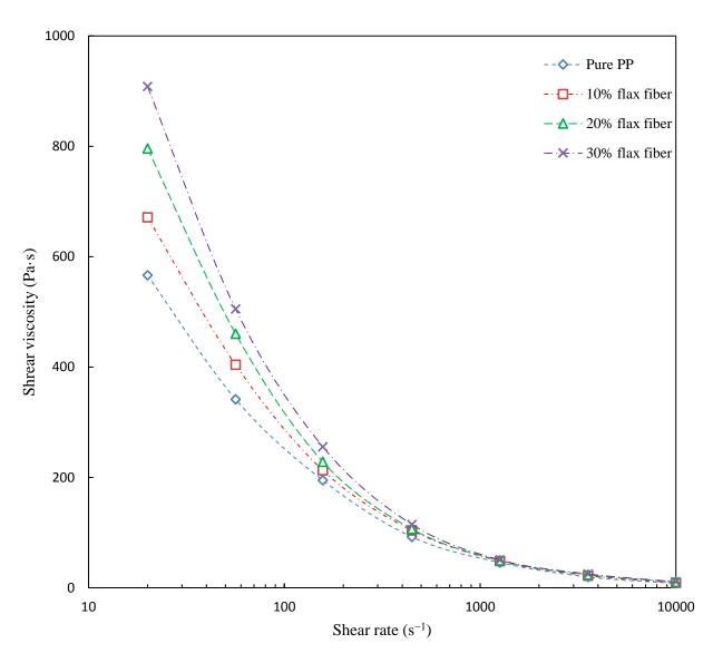
Fig. 4.5 Shear viscosity of pure PP and biocomposites at 230 °C as a function of the shear rate.
