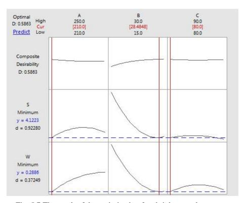
Fig. 5.7 The result of the optimization for shrinkage and warpage.
