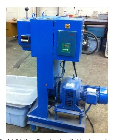
Fig. 3.4 Grinding mill machine for pelletizing the extrudates.
