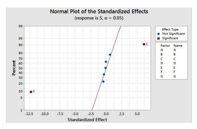
Fig. 5.6 Normal Plot of standardized effects for shrinkage.
