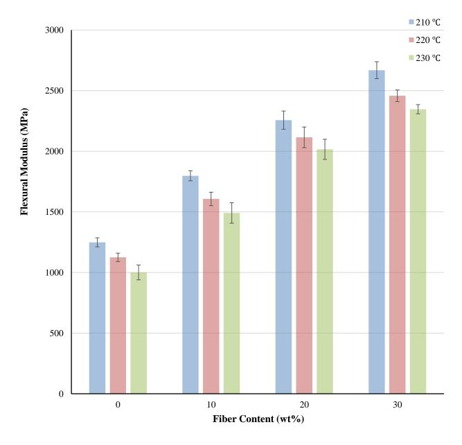
Fig. 3.20 The variation of flexural modulus of biocomposites with fiber contents and injection temperatures at injection pressure = 5.9 MPa.
