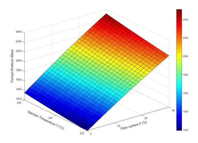
Fig. 3.16 The variation of Young's modulus of biocomposites with flax fiber content and injection temperature by the predicted model of Young's modulus.
