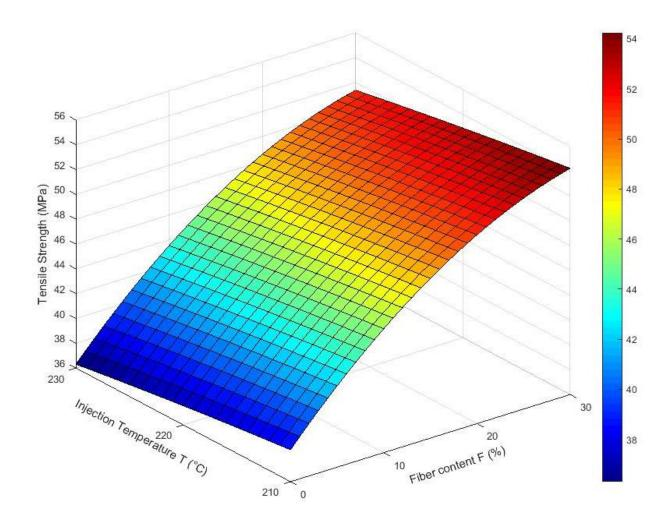
Fig. 3.15 The variation of tensile strength of biocomposites with flax fiber content and injection temperature by the predicted model of tensile strength.
