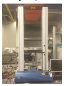
Fig. 3.8 Instron testing machine 3366 (Instron Corp., Canton, MA, USA).
