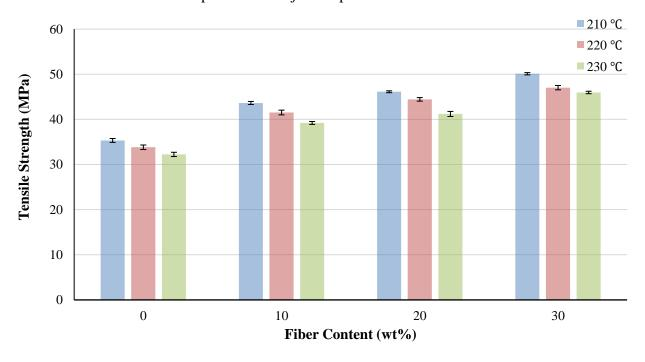
Fig. 3.11 The variation of tensile strength of biocomposites with fiber contents and injection temperatures at injection pressure 7.0 MPa.
