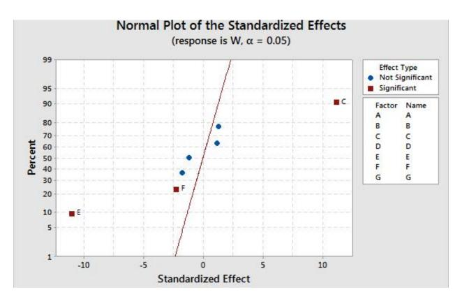
Fig. 5.4 Normal Plot of standardized effects for warpage.
