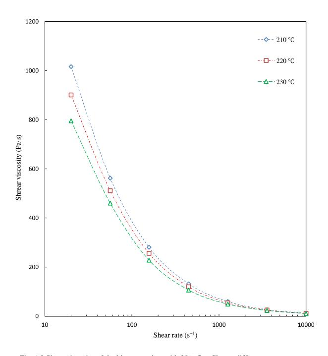
Fig. 4.8 Shear viscosity of the biocomposites with 20% flax fiber at different temperatures.
