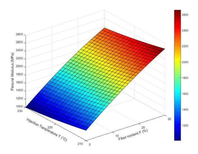
Fig. 3.24 The variation of flexural modulus of biocomposites with flax fiber content and injection temperature by the predicted model of flexural modulus.
