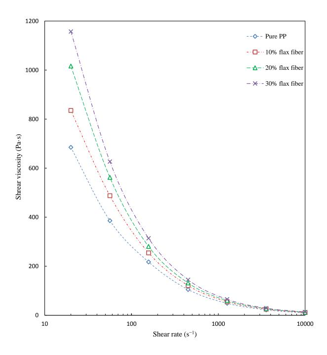
Fig. 4.3 Shear viscosity of pure PP and biocomposites at 210 °C as a function of the shear rate.
