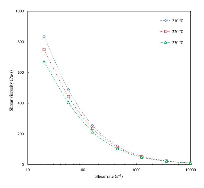
Fig. 4.7 Shear viscosity of the biocomposites with 10% flax fiber at different temperatures.
