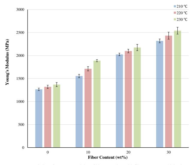
Fig. 3.13 The variation of Young's modulus of biocomposites with fiber contents and injection temperatures at injection pressure 5.9 MPa.
