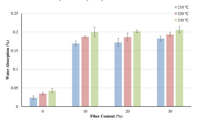
Fig. 3.27 The variation of water absorption of biocomposites with fiber contents and injection temperatures at injection pressure = 7.0 MPa.
