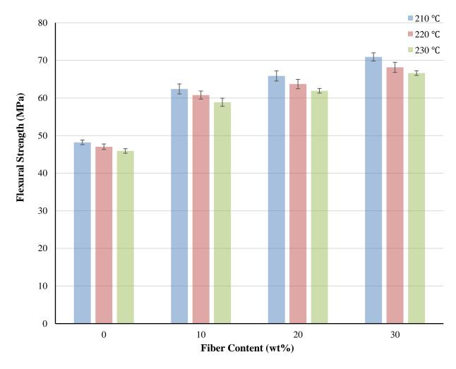
Fig. 3.19 The variation of flexural strength of biocomposites with fiber contents and injection temperatures at injection pressure = 5.9 MPa.
