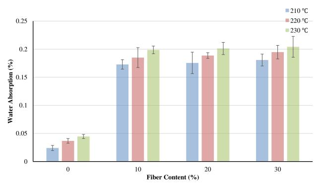
Fig. 3.26 The variation of water absorption of biocomposites with fiber contents and injection temperatures at injection pressure = 5.9 MPa.
