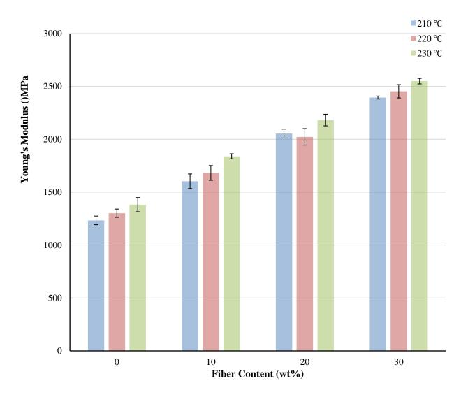
Fig. 3.14 The variation of Young's modulus of biocomposites with fiber contents and injection temperatures at injection pressure 7.0 MPa.
