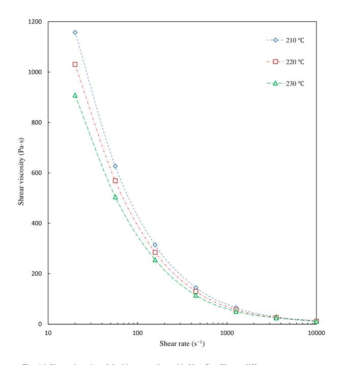
Fig. 4.9 Shear viscosity of the biocomposites with 30% flax fiber at different temperatures.
