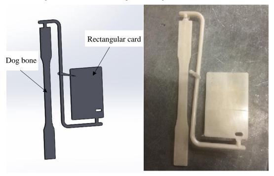
Fig. 3.7 Molded biocomposite product by injection molding (Dog bone is for tensile and flexural testing. Rectangular card is for water absorption testing).
