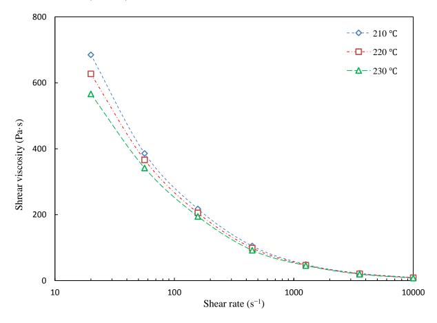
Fig. 4.6 Shear viscosity of pure PP at different temperatures.
