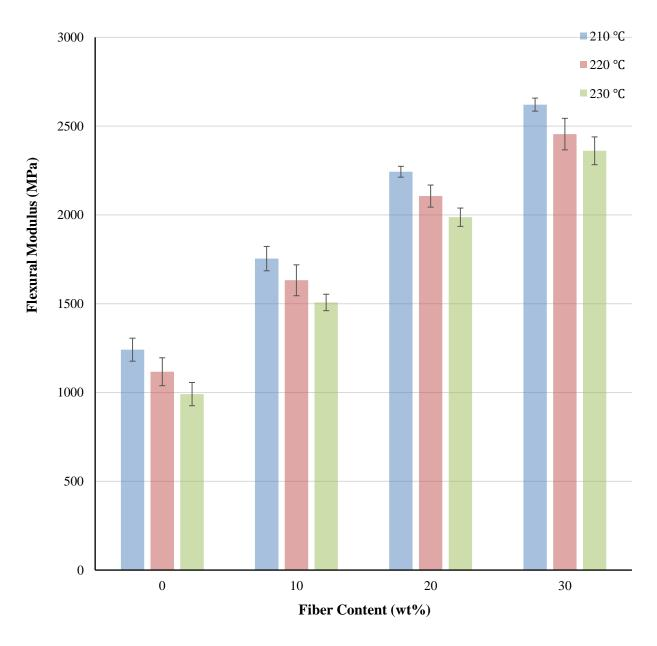
Fig. 3.18 The variation of flexural modulus of biocomposites with fiber contents and injection temperatures at injection pressure = 4.8 MPa.
