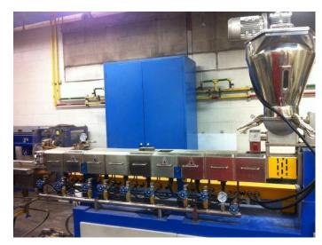
Fig. 3.2 Twin-screw extruder for compounding the mixture.
