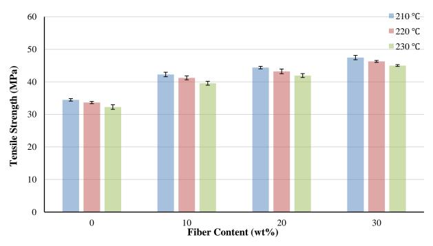
Fig. 3.9 The variation of tensile strength of biocomposites with fiber contents and injection temperatures at injection pressure 4.8 MPa.
