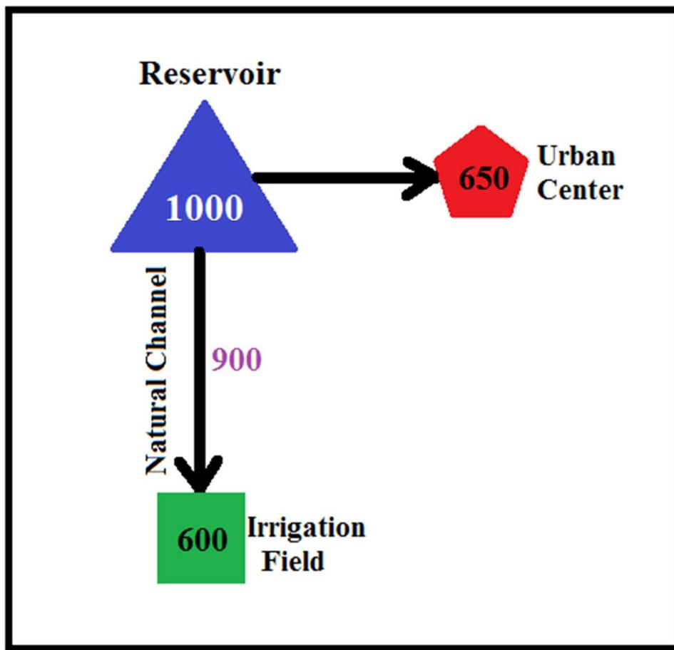
Figure 3.5: Simple water system to explain WRMM operation procedure
