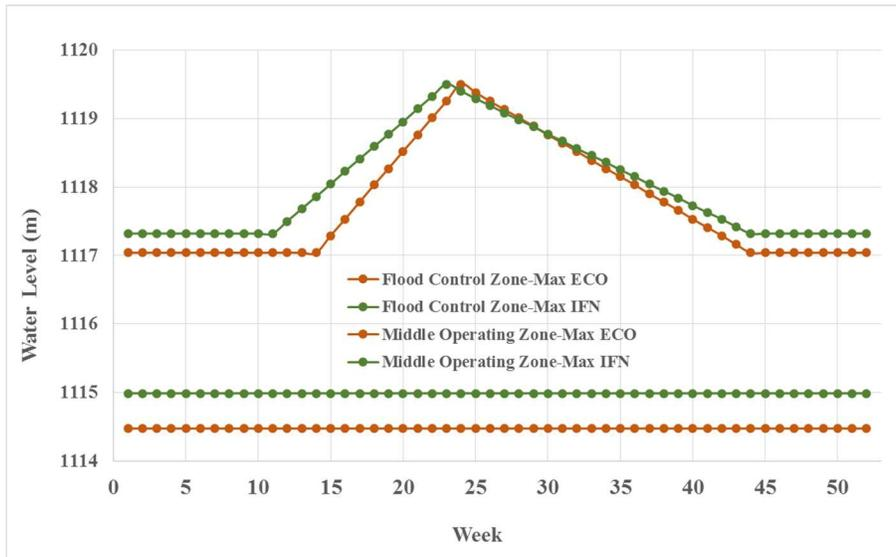
Figure 4.34: Operating zones causing the maximum economic benefit (orange curves) and the maximum water allocated to IFN (green curves) on the PFEI
