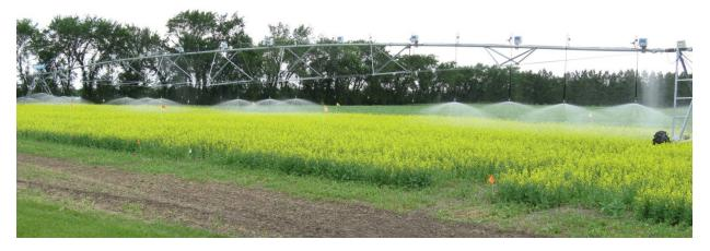
Figure 3. VRI system in use to irrigate plots separately within an irrigation study.
