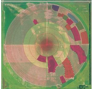
Figure 2. Diagram showing 5400 irrigation management zones in a field with VRI, and a prescription to vary irrigation amounts in areas of special soil types and research trials.
