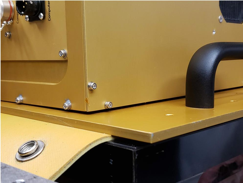
**Figure 4.4:** A gap between the Electronics Box and baseplate, due to bolt stretching caused by the shock of landing.
