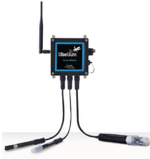
Figure 1.6. Libelium Waspote Plug & Sense sensor device (from Libelium Technical guide, 2018).
